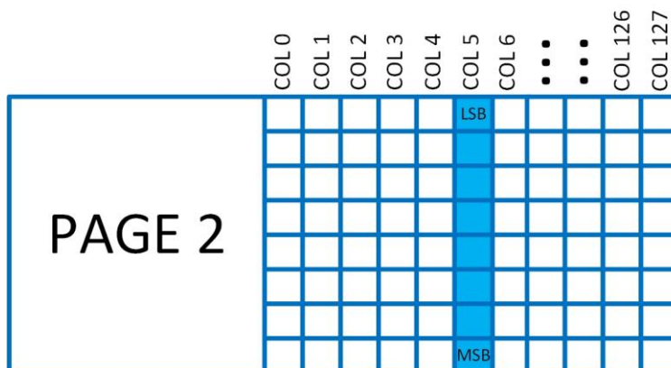
Figure 6. SSD1306 Single Byte Representation
