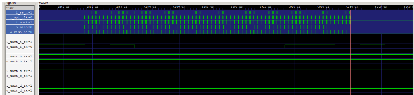
Figure 8. Communication with the Converter via SPI
