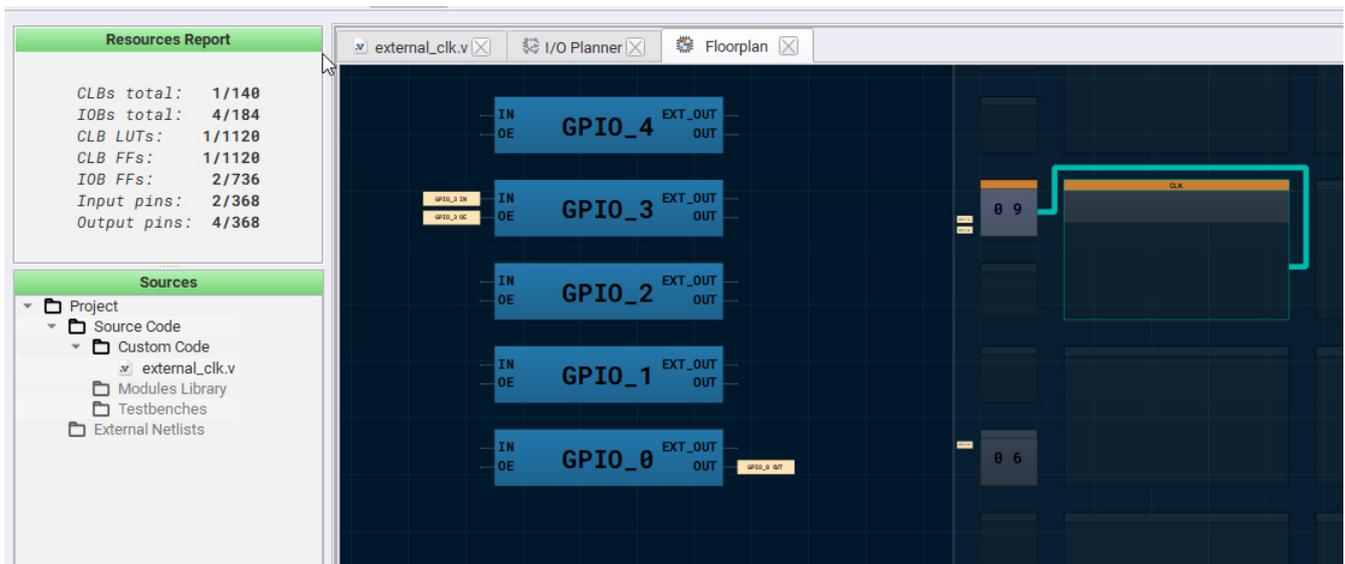
Figure 1: Floorplan & CLB Utilization
