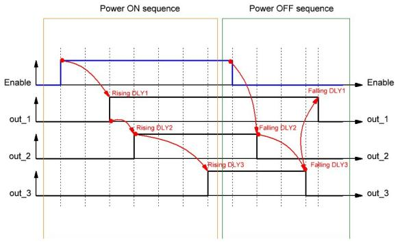
Figure 4: Power Sequencing Output Waveform
