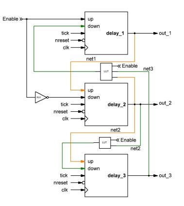
Figure 3: Power Sequencing Block Diagram
