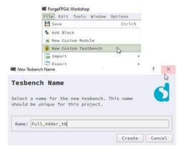
Figure 2: Steps to Launch Custom Testbench
