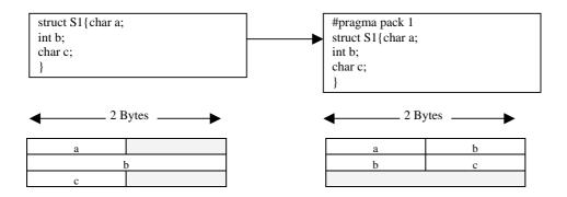
As the structure is packed, integer b will not be aligned. This will improve the RAM size but operational speed will be degraded, as the access of 'b' will take up two cycles.
