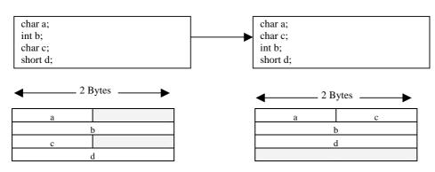
Alternatively programmers can set the setting in HEW Options  $\rightarrow$  H8 Toolchain  $\rightarrow$  C/C++  $\rightarrow$  Other  $\rightarrow$  "Group data by alignment", and the compiler will "rearrange" to group similar type of variables together.
