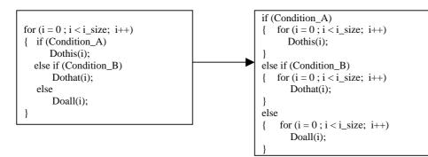
For the first case, Condition\_B will have an overhead of the "if(Condition\_A)".
