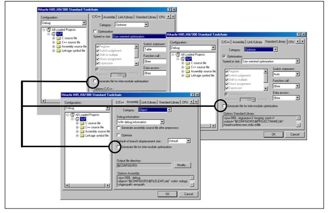
This will enable inter -module optimizing information to be generated for the linker to perform a better optimization.
