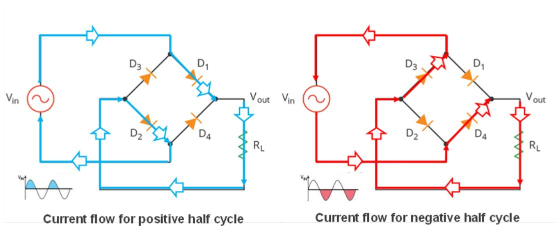
**Figure 2-2 Current flow in Full Bridge rectifier**
