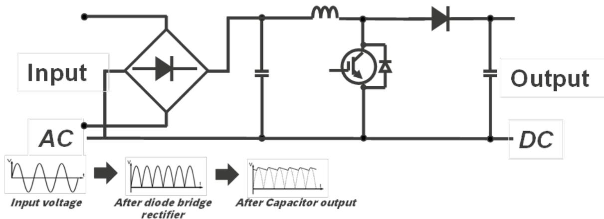
Figure 3-1 Active Power Factor Correction with switching
