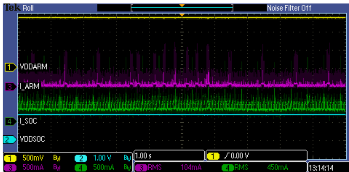
Figure 6: BYPASS MODE (I do_active =OFF) at 1GHz – Voltage Rails and System Current
