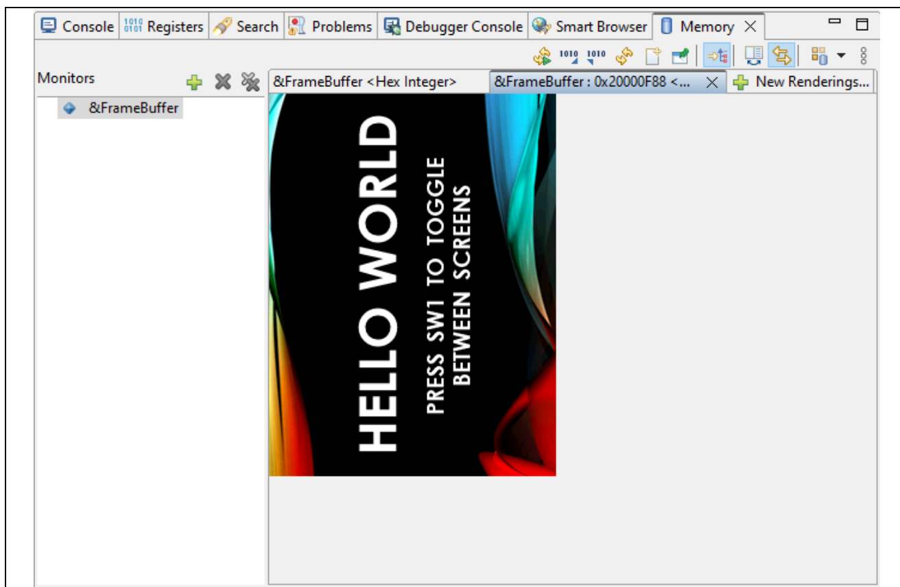
Figure 37. Raw image rendering of the FrameBuffer pixel array in RAM
