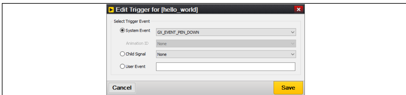
Figure 22. The defined system trigger event for the hello_world screen is GX_EVENT_PEN_DOWN
