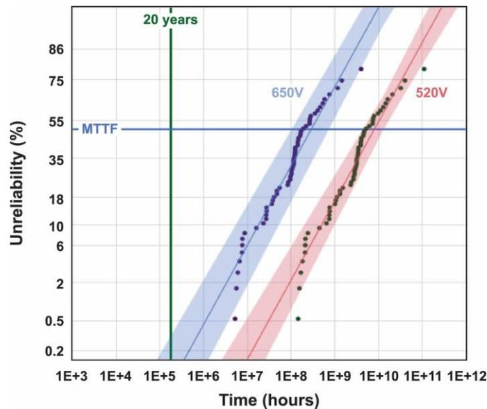
Figure 4. “Use-plots” based on voltage-accelerated testing showing all failed devices during HVOS testing at 82°C for the reciprocal field TDDb model. 99% confidence limits shown, Tj = 82°C, TDDb inverse voltage model (Smith, 2015)
