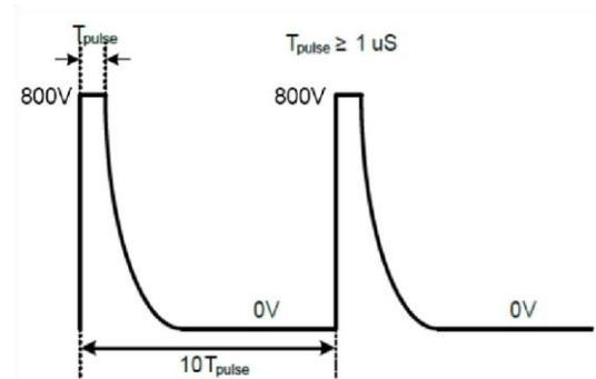
Figure 6. Spike voltage waveform
