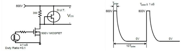
Figure 5. Spike voltage test circuit
