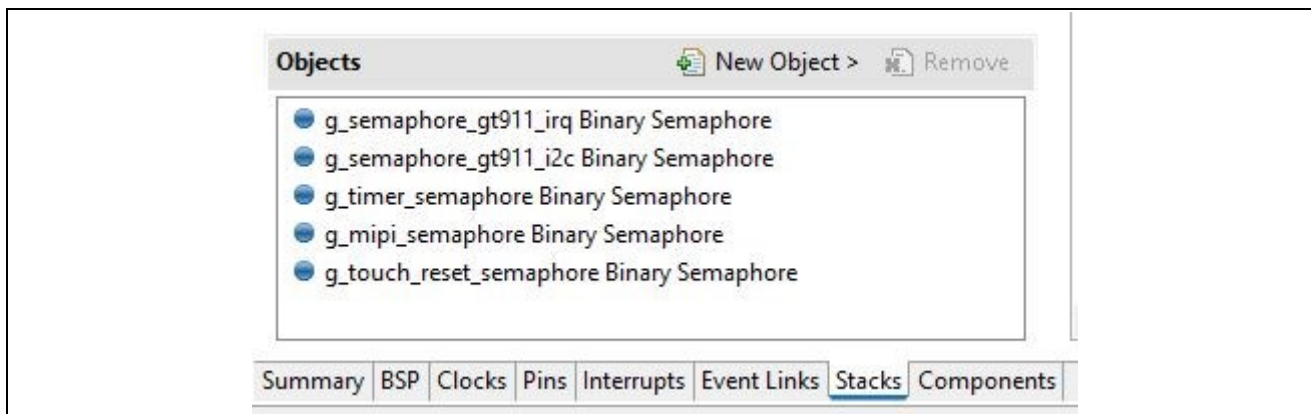
Figure 30. The FreeRTOS semaphore objects used by the thermostat graphics application
