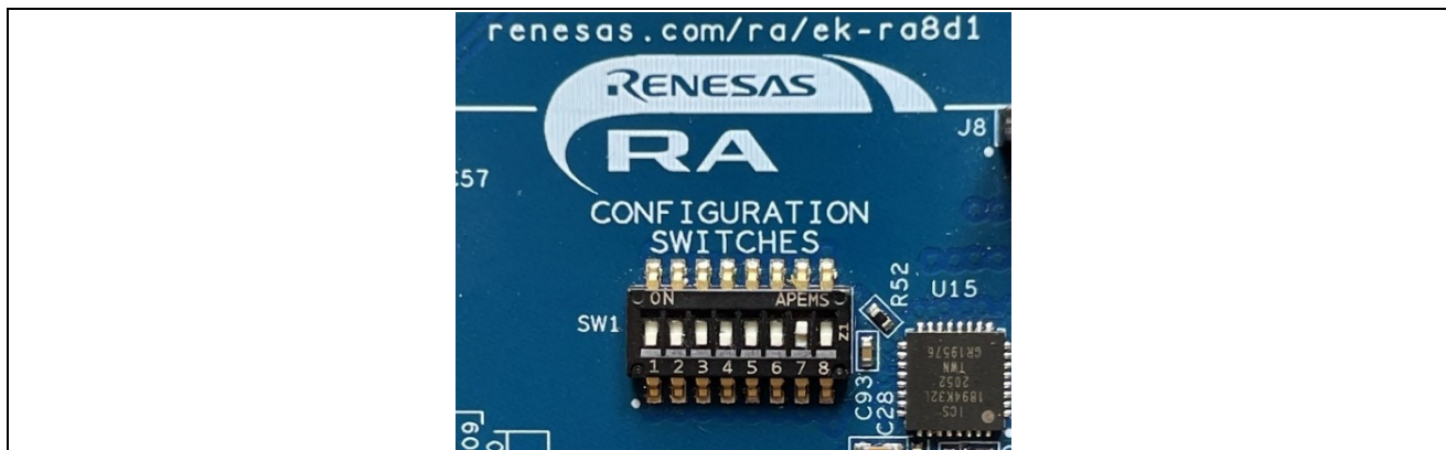
Figure 36. Enabling SW1-7 for SDRAM on the EK-RA8D1
