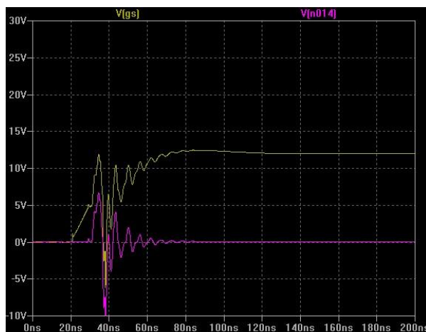
Figure 9: simulation showing voltage on the internal source node.
