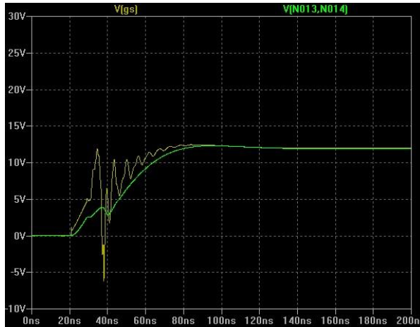
Figure 10: simulation showing internal V_{gs}
