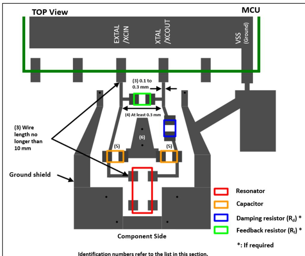
Figure 19. Example of the EXTAL/XCIN and XTAL/XCOU Routing Pattern: LQFP Package
