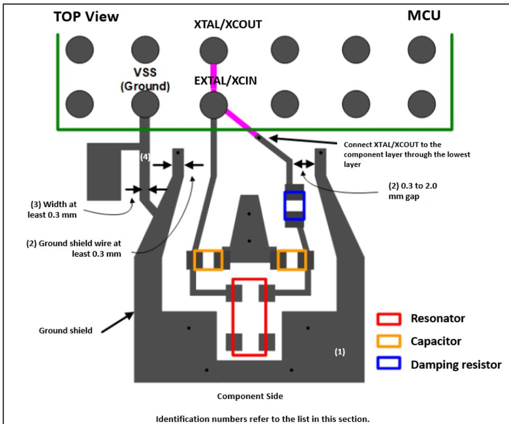
Figure 24. Example of the ground shield tracing: LGA Package
