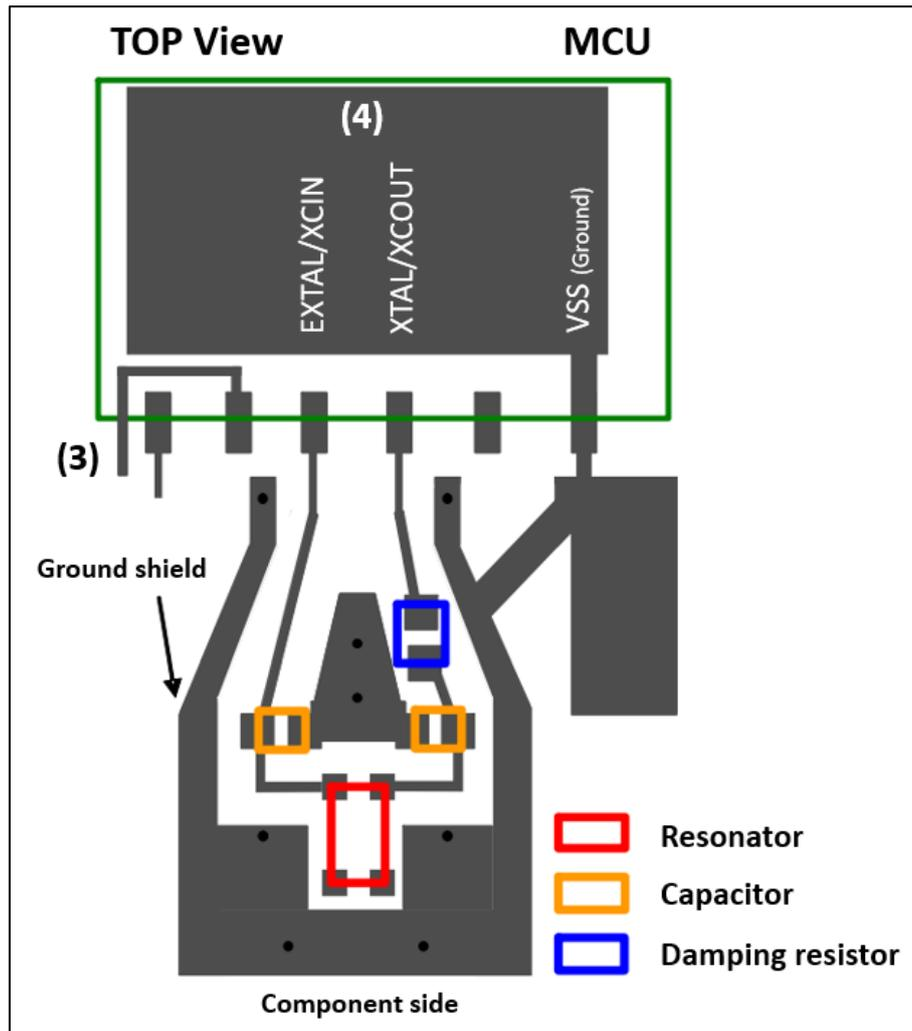
Figure 31. Example of Routing for Other Points: LQFP Package
