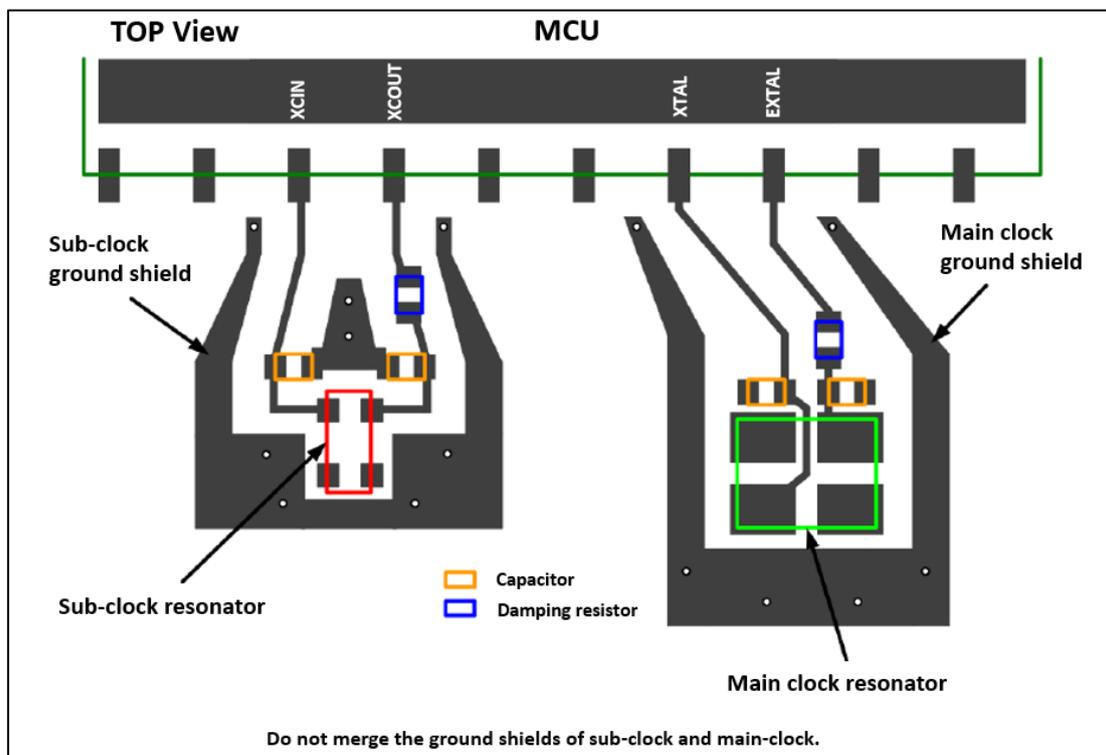
Figure 26. Example of the main clock and sub-clock ground shield configuration
