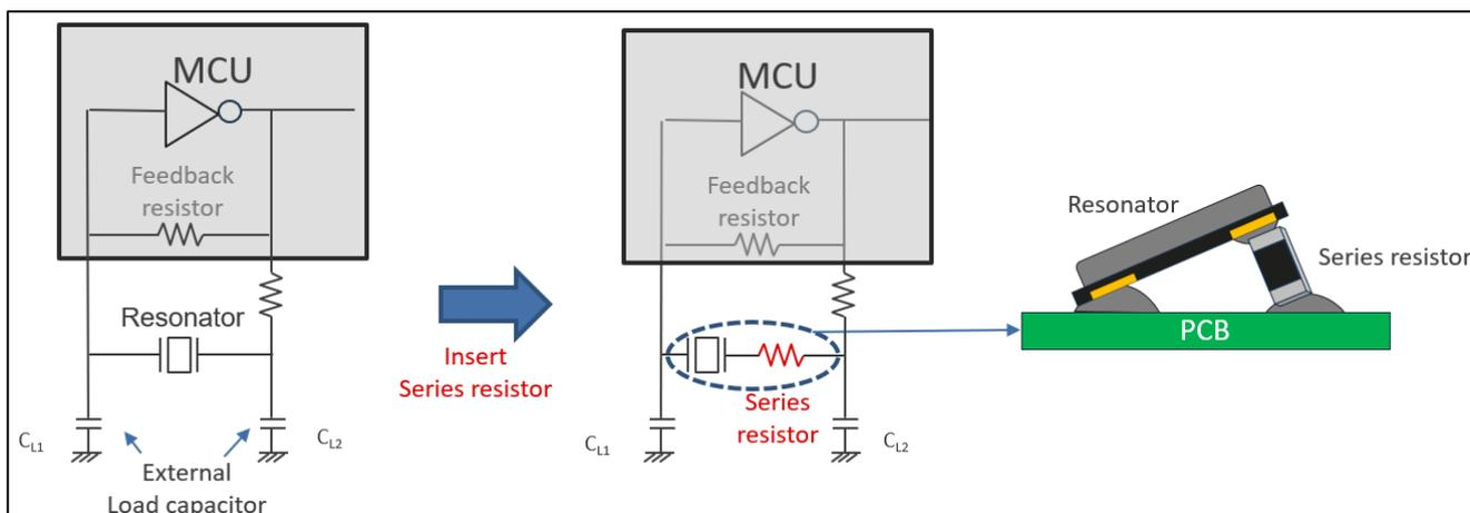
Figure 15. Measurement method of the negative resistance
