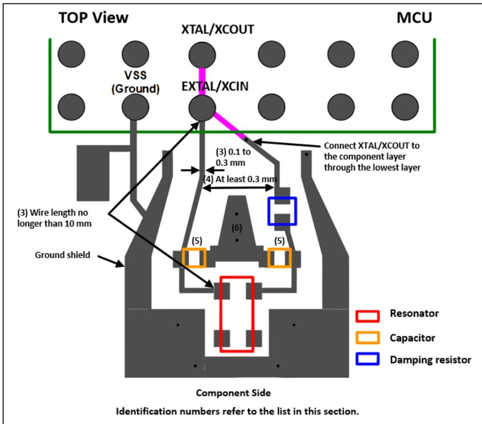
Figure 20. Example of the EXTAL/XCIN and XTAL/XCOOUT Routing Pattern: LGA Package
