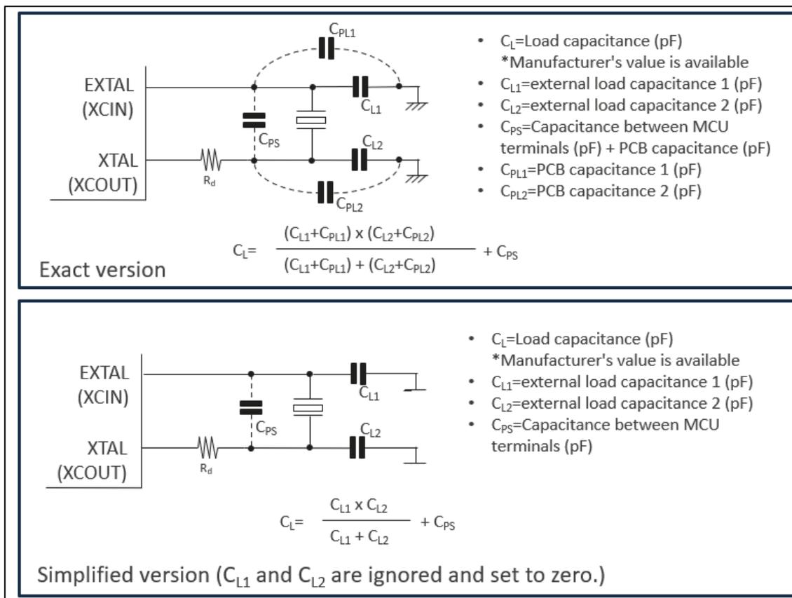
Figure 18. Formula for the External Load Capacity ( $C_{L1}$  and  $C_{L2}$ )
