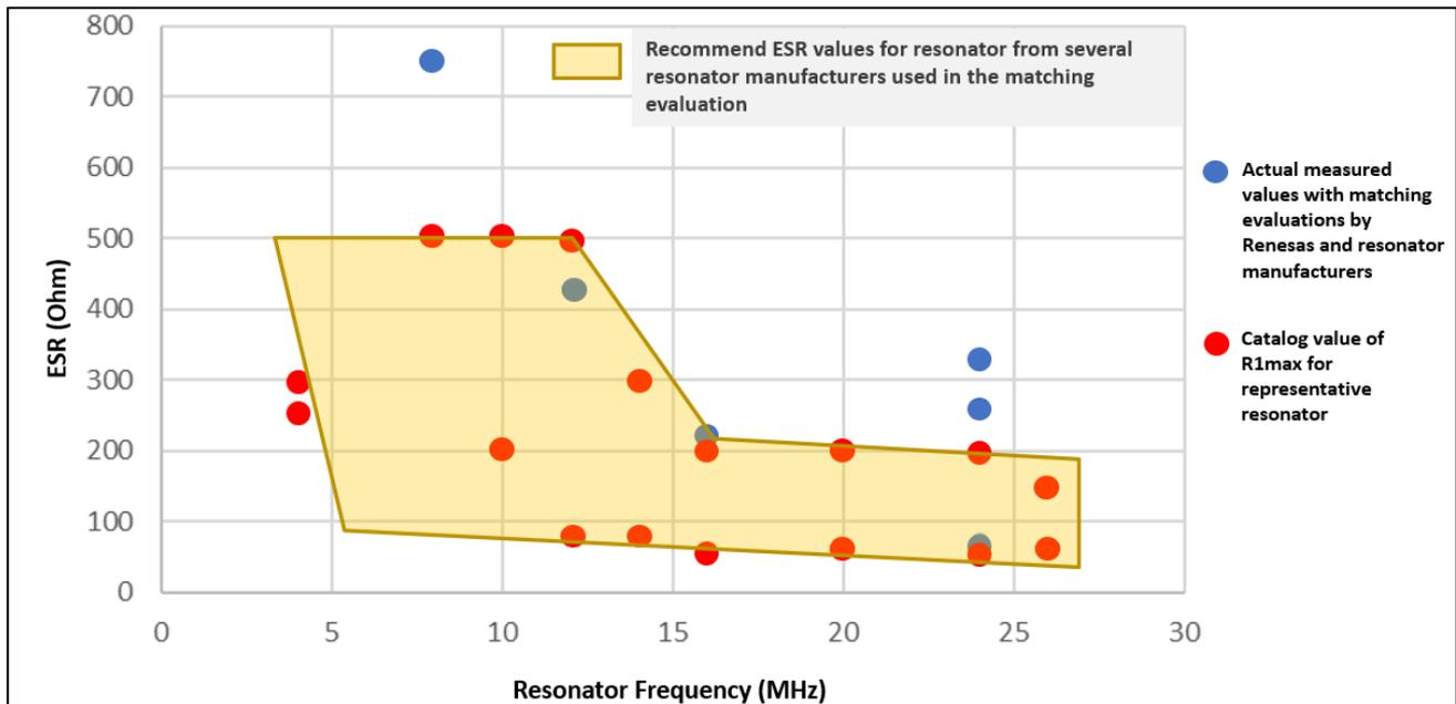
**Figure 2. Group 1, Main clock: Resonator Frequency vs ESR max**
