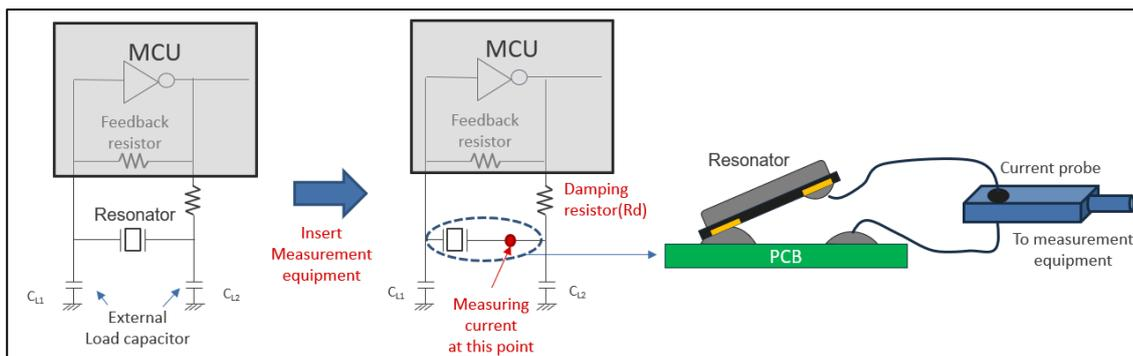
Figure 16. Measurement method of the oscillations excitation power
