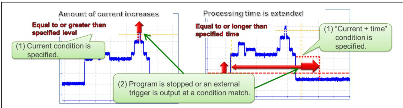
Figure 1-2 Detection in Detail
