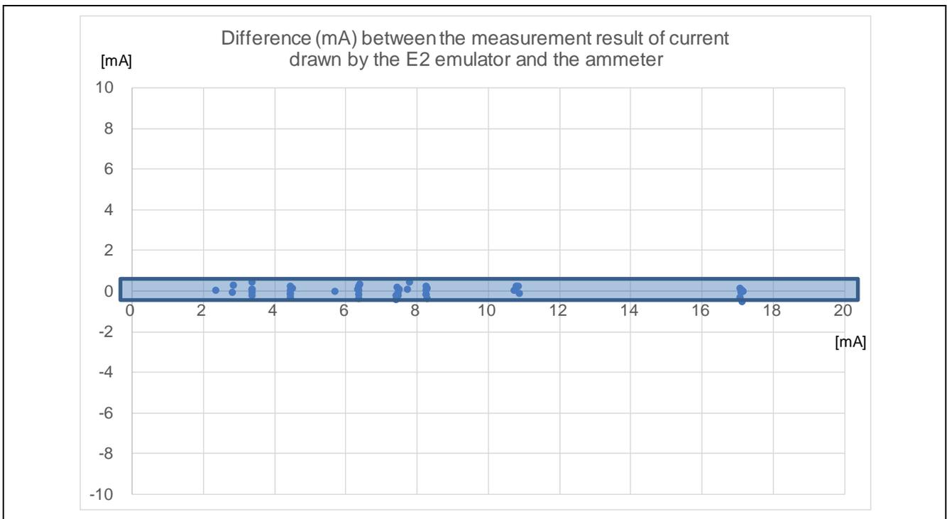
Figure 5-4 Difference between the Measurement Result of Current Consumption and the Ammeter (2)
