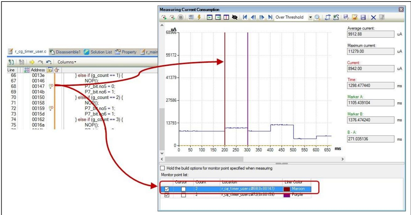
Figure 4-19 Link between Monitoring Point and Program
