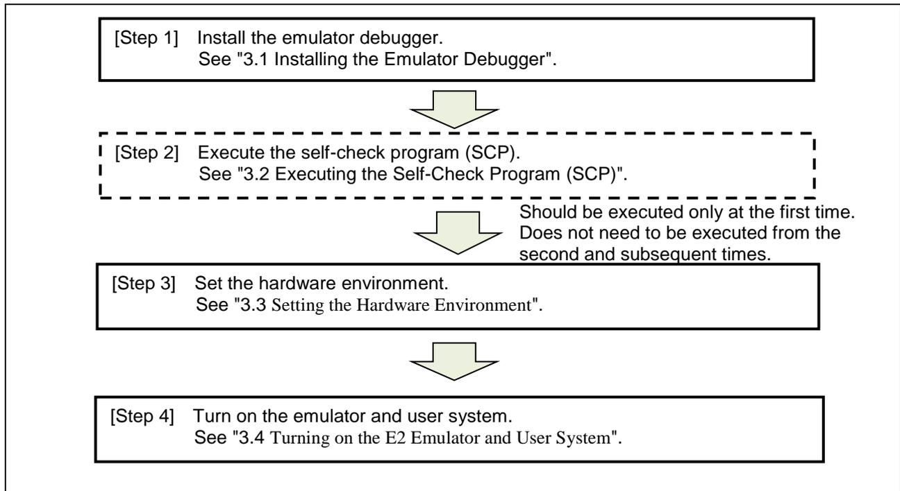
Figure 3-1 Setup Procedure
