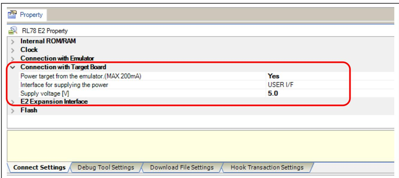
Figure 4-1 Connection Settings of E2 Emulator Debugger
