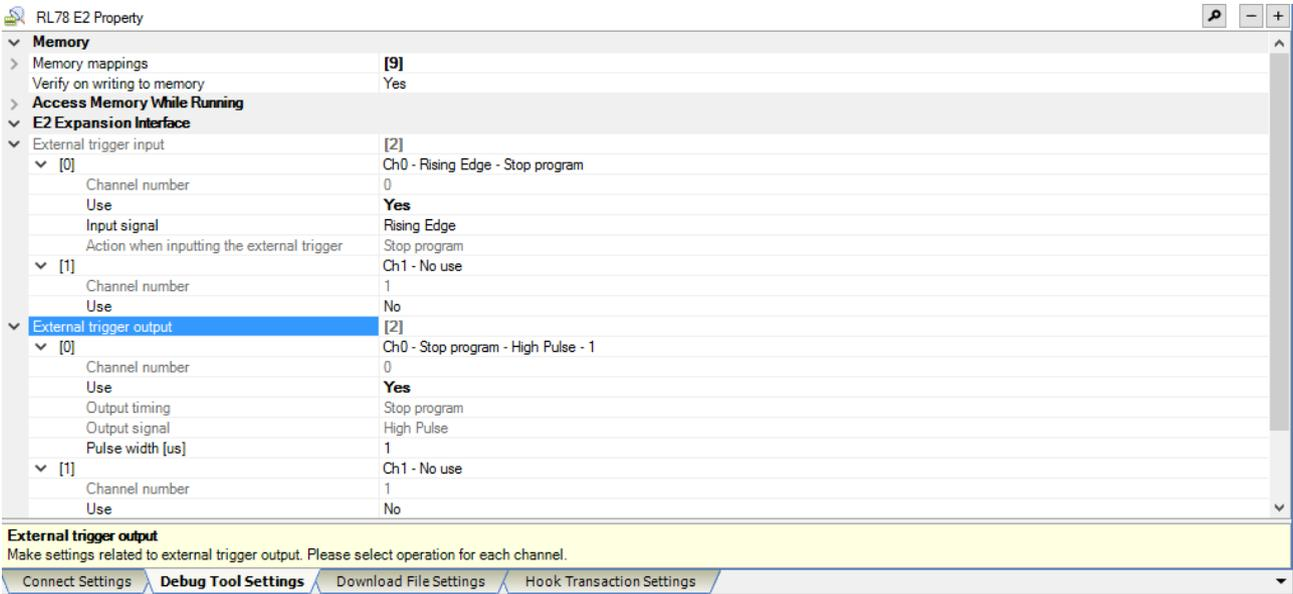
The screenshot shows the 'RL78 E2 Property' dialog box. The 'E2 Expansion Interface' section is expanded. Under 'External trigger output', channel 0 is selected. The settings for channel 0 are: Channel number 0, Use Yes, Output timing Stop program, Output signal High Pulse, and Pulse width [us] 1. Channel 1 is set to 'No use'.
