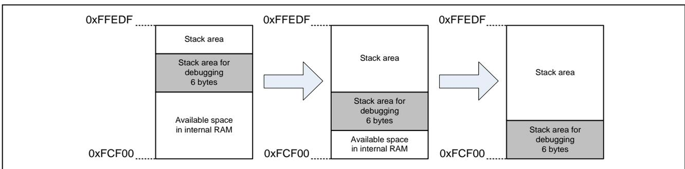
**Figure 2-1 Variation of Address of Stack Area for Debugging**
