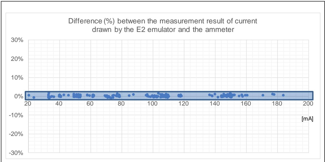
Figure 5-3 Difference between the Measurement Result of Current Consumption and the Ammeter (1)
