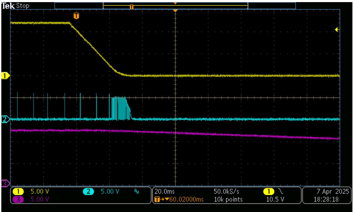
Figure 35. Shutdown via Falling V_{IN} , 10 mA Load. Ch.1 = V_{IN} , Ch.2 = Q1 V_{GS} , Ch.3 = V_{OUT}
