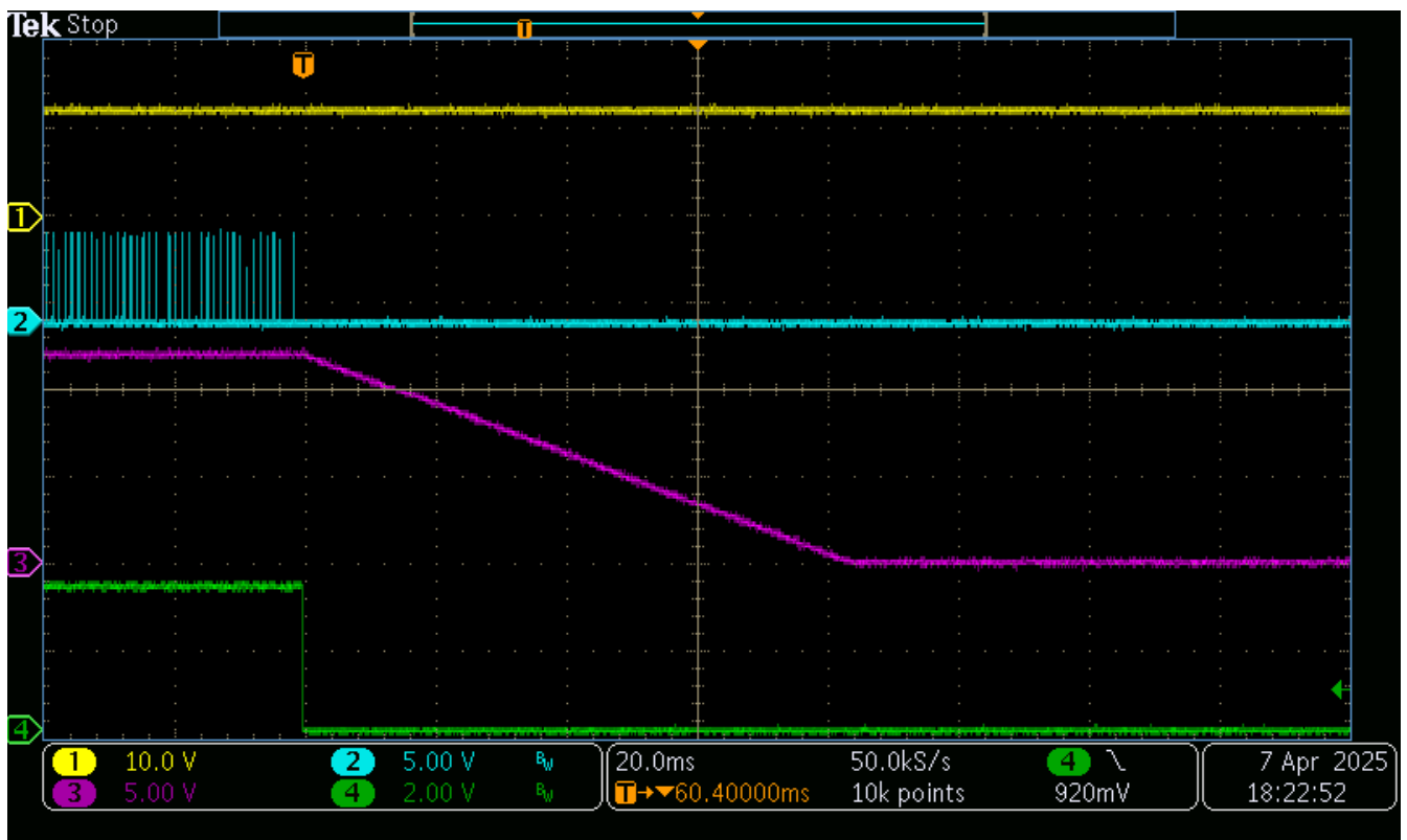
Figure 33. Shutdown via EN/SD*, 10 mA Load. Ch.1 = V_{IN} , Ch.2 = Q1 V_{GS} , Ch.3 = V_{OUT} , Ch.4 = EN/SD*
