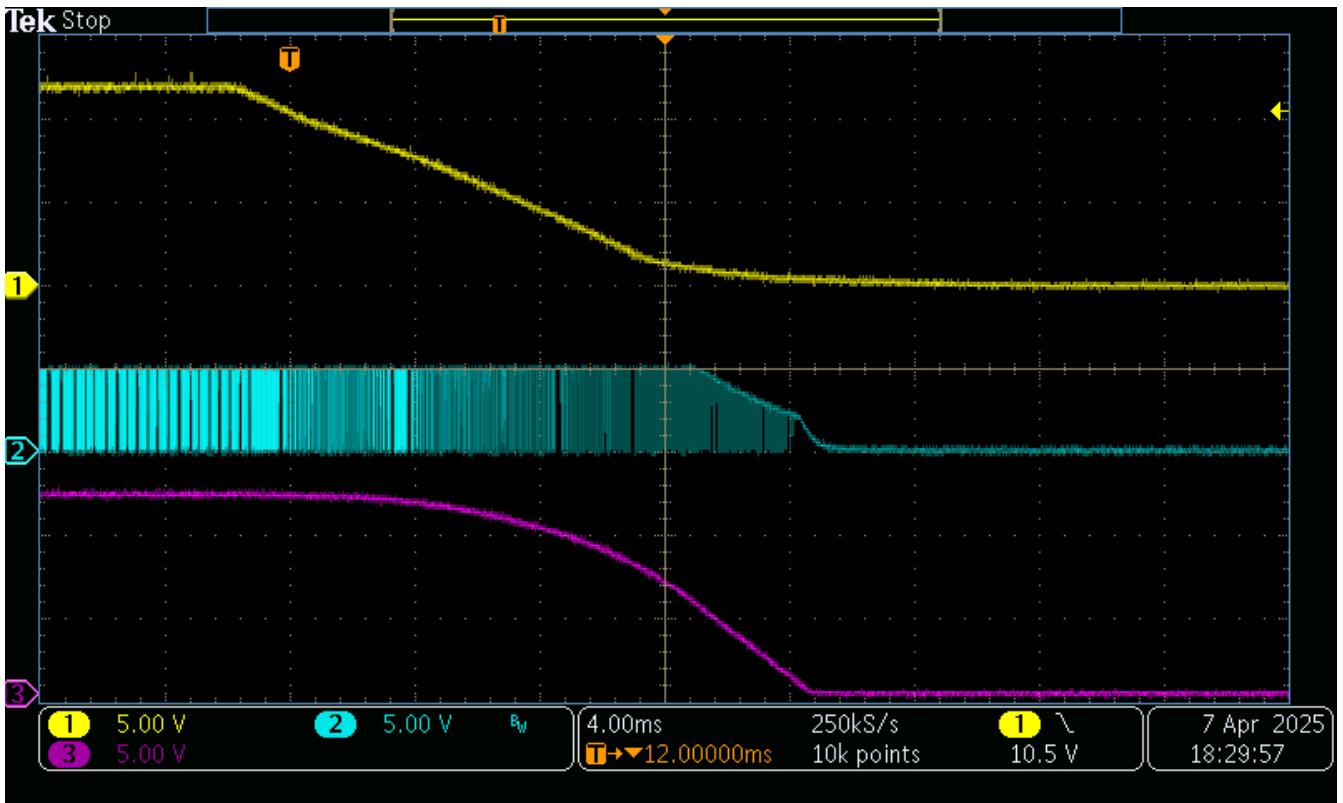
Figure 36. Shutdown via Falling V_{IN} , 1 A Load. Ch.1 = V_{IN} , Ch.2 = Q1 V_{GS} , Ch.3 = V_{OUT}
