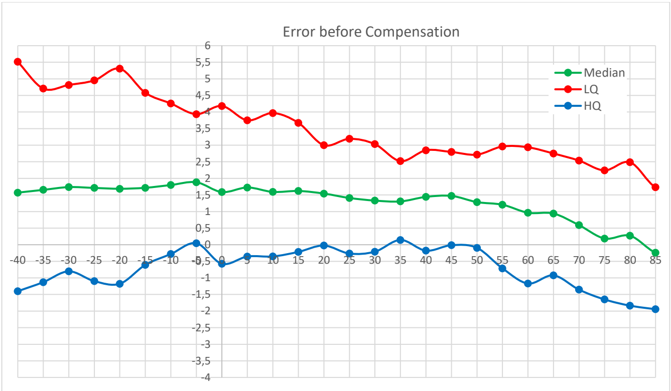
Figure 5. Temperature Sensor Error before Compensation
