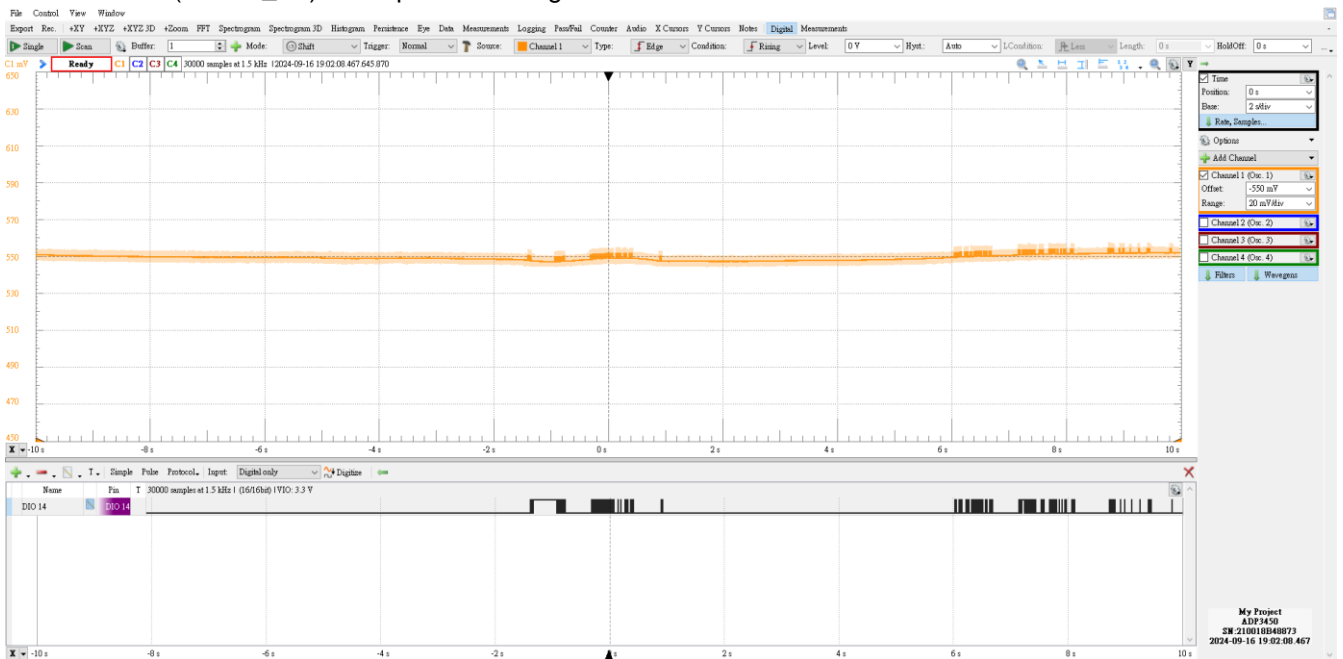
Figure 11. PIR signal measurement at 2 meters
