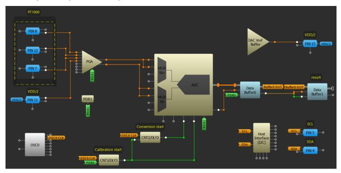
Figure 2. PT1000 Interface AnalogPAK Design
