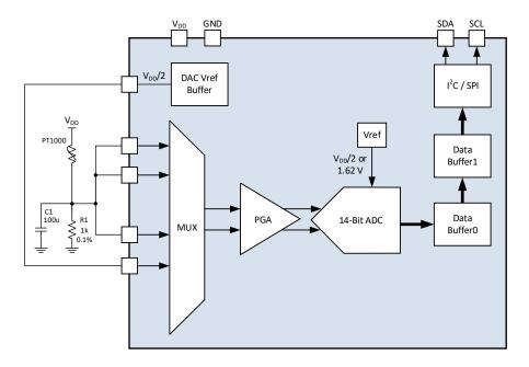
Figure 1. PT1000 Interface Simplified Block Diagram
