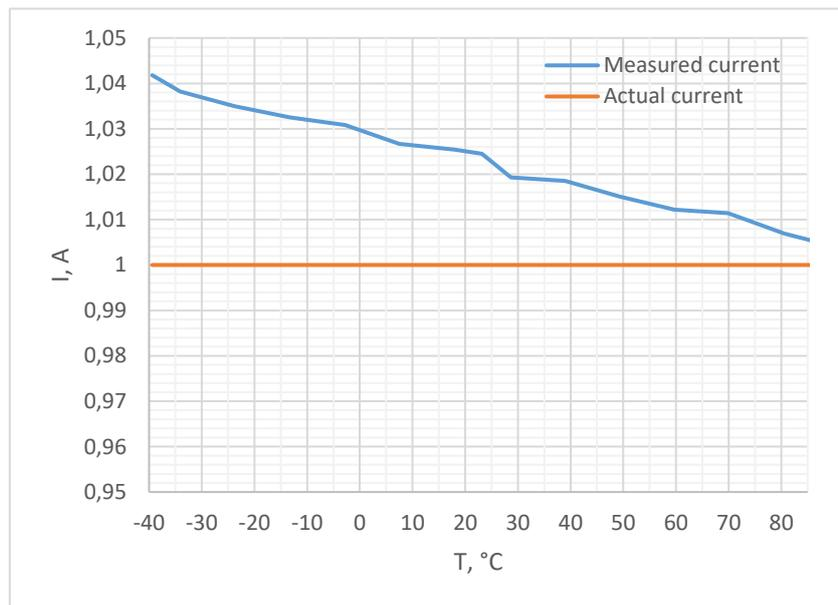
Figure 7. Measured current vs Temperature, 1 A, Gain 64x
