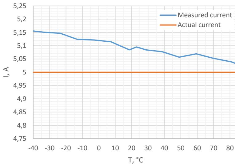
Figure 10. Measured Current vs Temperature, 5 A, Gain 8x
