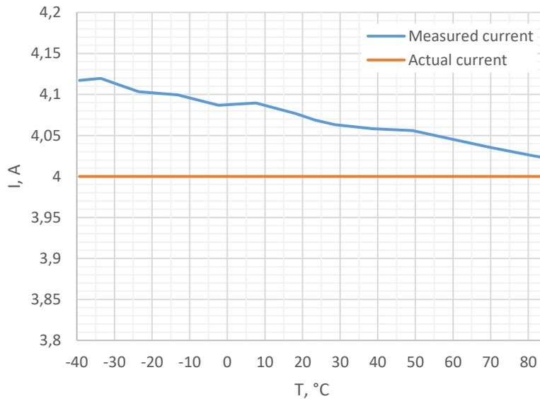
Figure 9. Measured Current vs Temperature, 4 A, Gain 16x
