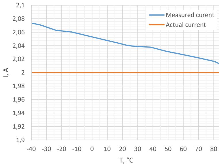
Figure 8. Measured current vs Temperature, 2 A, Gain 32x
