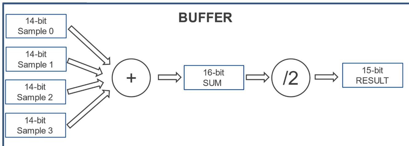
Figure 1. Oversampling Block Diagram in SLG47011 Data Buffer
