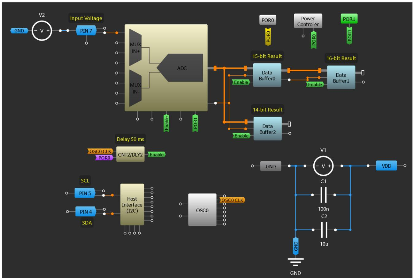
**Figure 2. Go Configure Schematic of ADC Oversampling**
