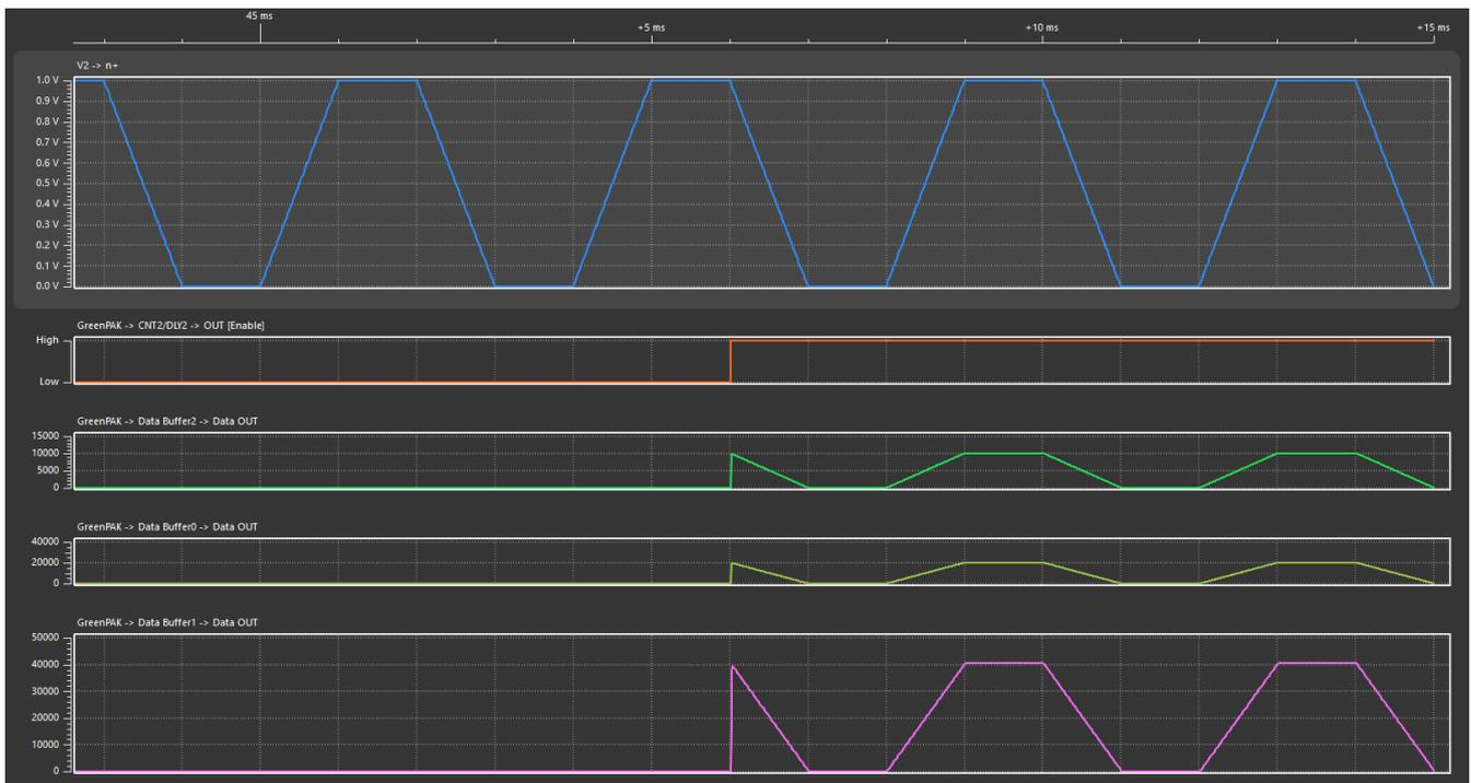
Figure 4. Simulation Waveforms Illustrating ADC Oversampling
