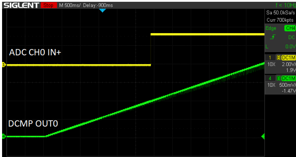
Figure 2. Waveform Illustrating Overvoltage Monitor
