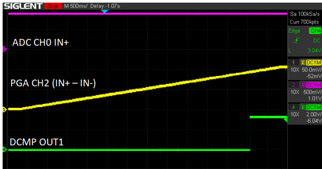
Figure 4. Waveform Illustrating Overpower Monitor
