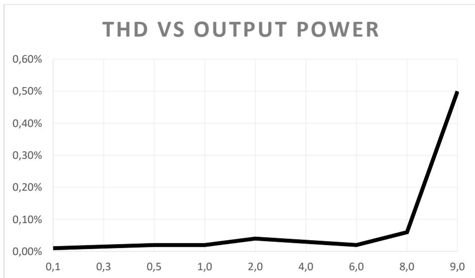
Figure 7: THD vs Output Power,  $R_L = 8 \text{ Ohm}$ ,  $f = 1 \text{ kHz}$
