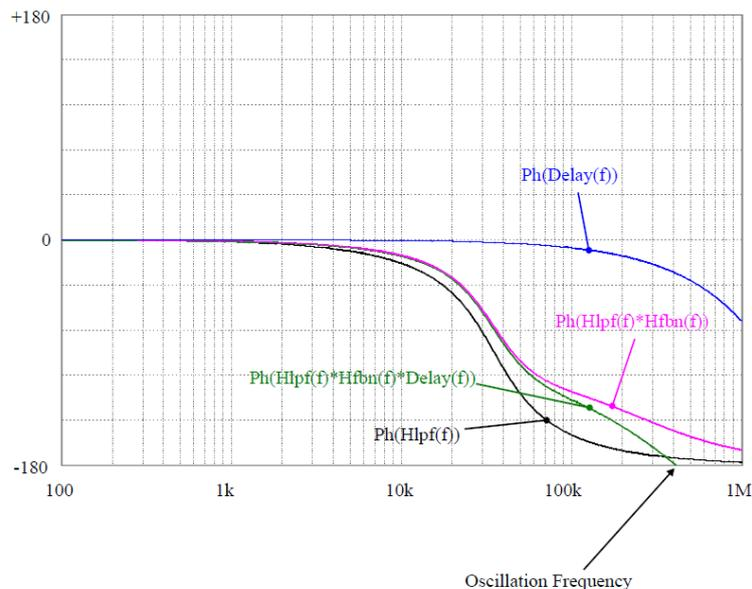
Where  $H_{lpf}$  is the transfer function of the LC filter and  $H_{fbn}$  that of the feedback network
