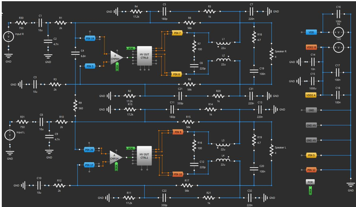
**Figure 5: Stereo Full-bridge UcD Audio Power Amplifier Project**
