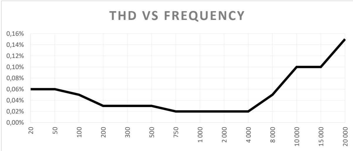
Figure 8: THD vs Frequency, RI = 8 Ohm, Pout = 1 W
