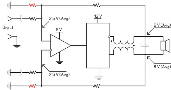
Figure 6: Simplified Circuit of the Amplifier. One Channel
