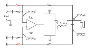
Figure 6: Simplified Circuit of the Amplifier. One Channel
