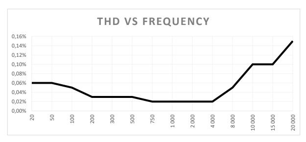
Figure 8: THD vs Frequency, RI = 8 Ohm, Pout = 1 W
