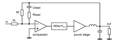
Figure 3: Phase-Shift Control Using the Reconstruction Filter Topology
