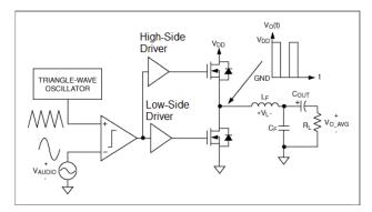
Figure 1: Half-Bridge Class D Amplifier, Basic Topology
