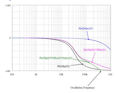
Where  $H_{lpf}$  is the transfer function of the LC filter and  $H_{fbn}$  that of the feedback network Delay(s) is a linear phase shift function representing the propagation delay.
