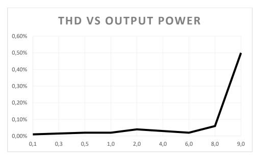
Figure 7: THD vs Output Power, RI = 8 Ohm, f = 1kHz
