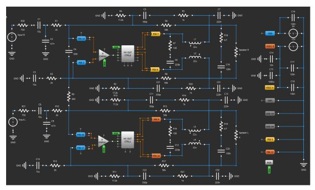
Figure 5: Stereo Full-bridge UcD Audio Power Amplifier Project
