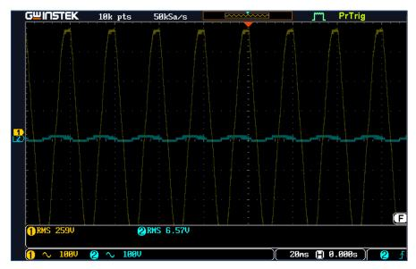
Figure 11: Overvoltage Condition
