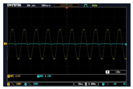
**Figure 13: Undervoltage Condition**
