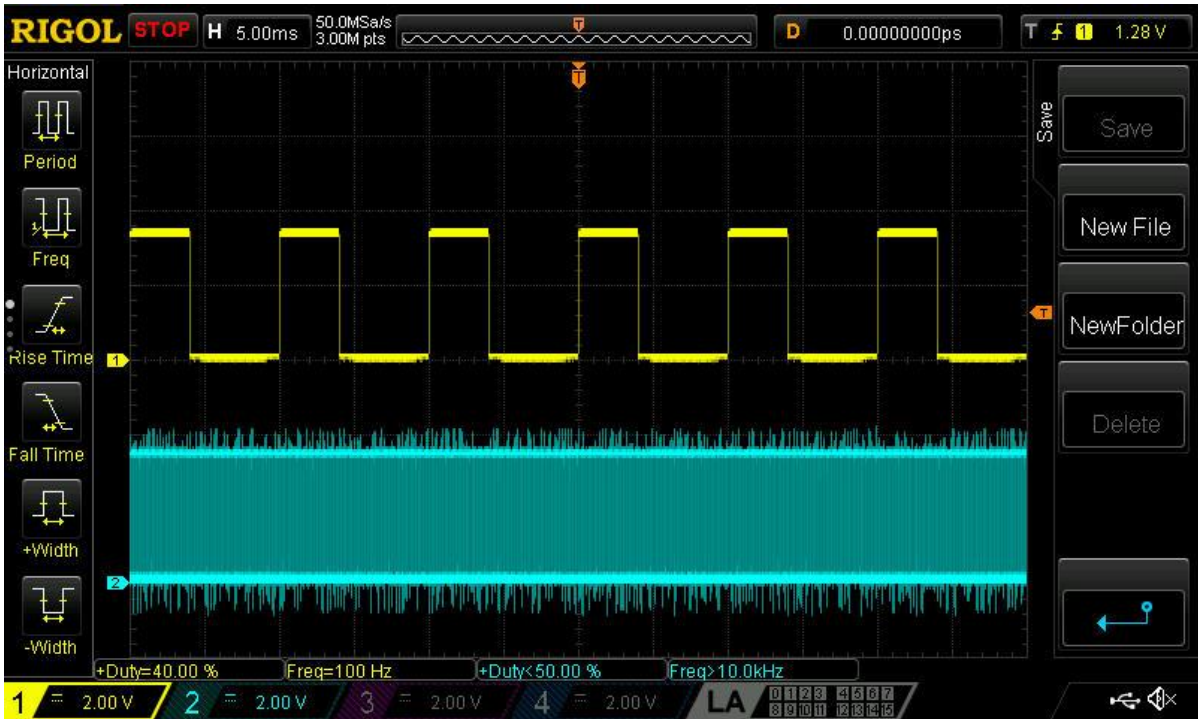
Figure 4: Shifting Input Frequency from 100 Hz to 7.81 kHz
