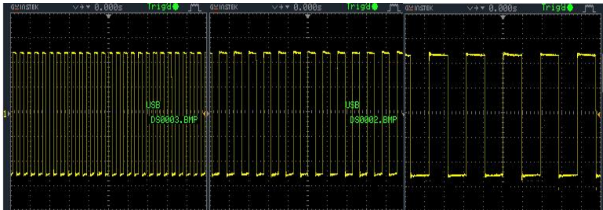
Figure 17: Output Waveform of Single-Phase Inverter
