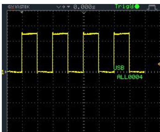
Figure 15: Switching Pattern for S1 and S4
