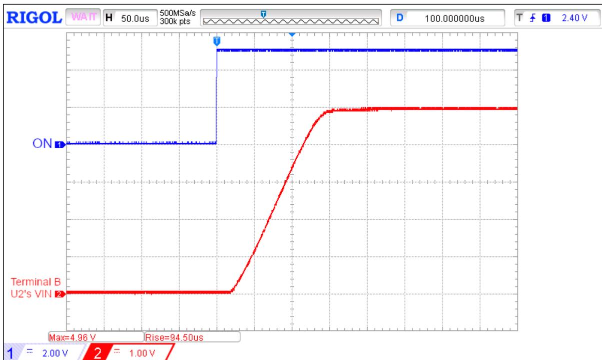
**Figure 3. BLS Turn-ON Operation for Two, Series-Connected SLG59M1558V GreenFET Load Switches for  $V_{\text{IN(A)}} = 5 \text{ V}$ ,  $R_{\text{LOAD}} = 20 \Omega$ ,  $C_{\text{LOAD}} = 10 \mu\text{F}$**
