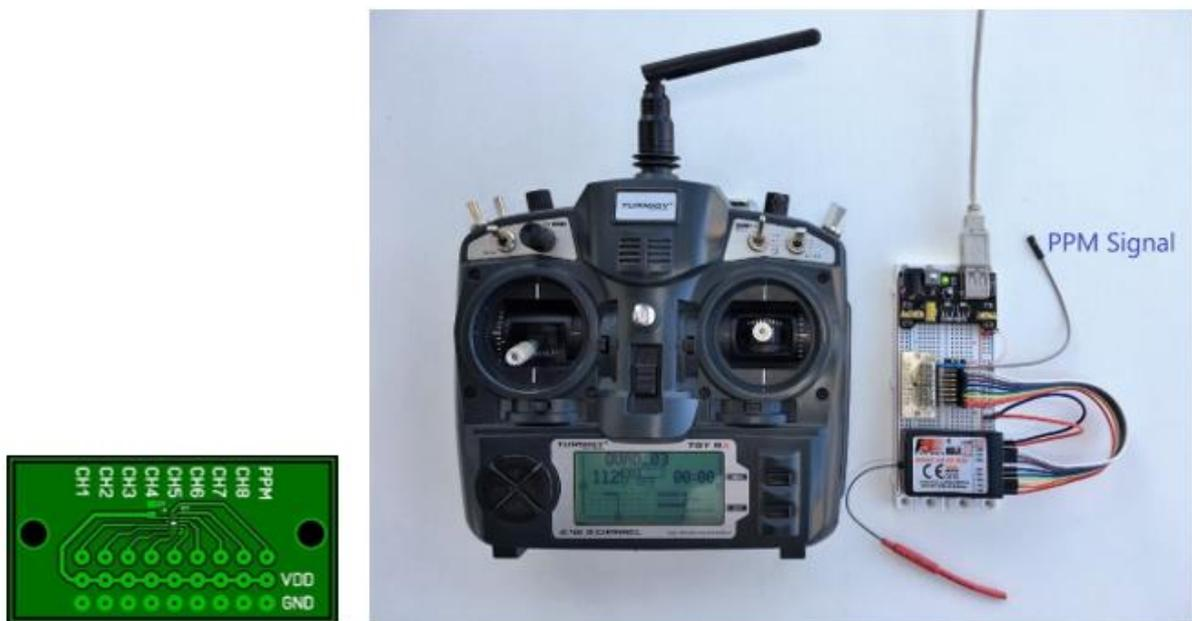
**Figure 4: Prototype PCB and Test Board**
