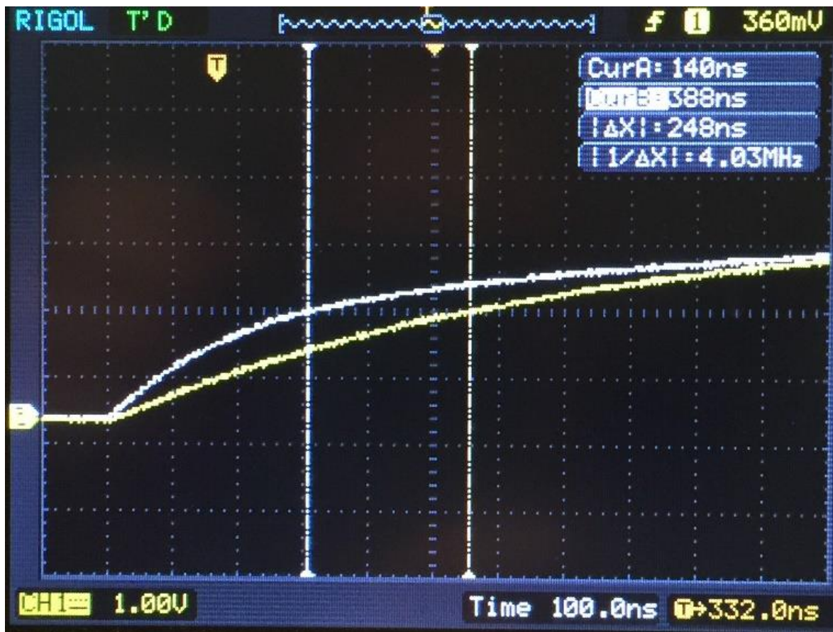
Figure 2: Oscilloscope Capture Showing the Difference in Risetime
