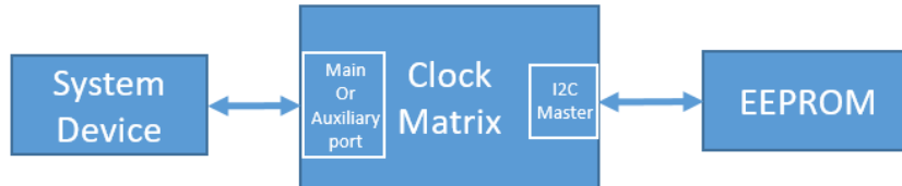
Figure 10. Programming the EEPROM through ClockMatrix
