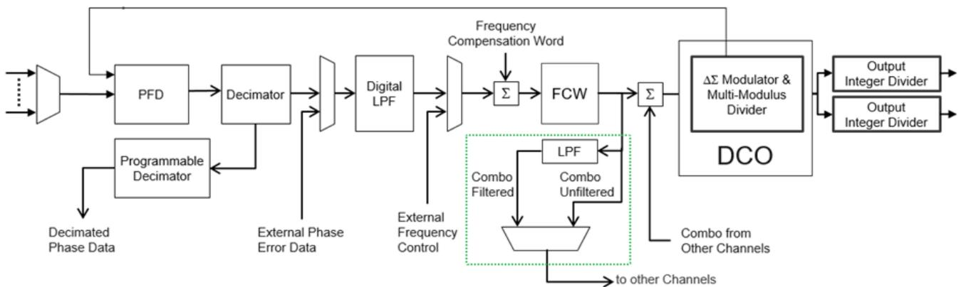
Figure 1. Block Diagram of One Channel of ClockMatrix
