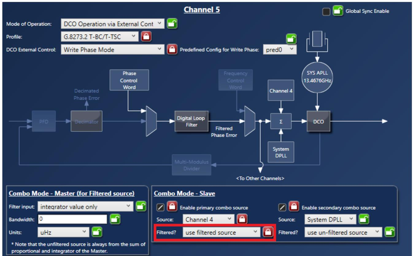
Figure 8. Filter Selection Combo Slave Settings as Shown in the GUI
