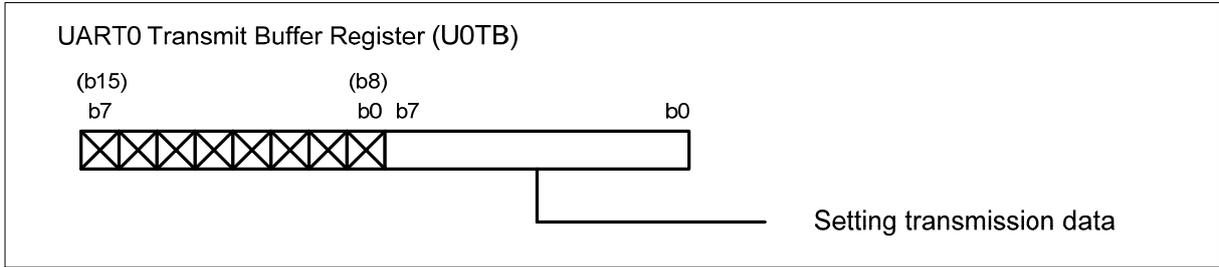
(7) Check UART0 Transmit/receive Control Register 1 to get the status of UART0 Transmit Buffer Register
