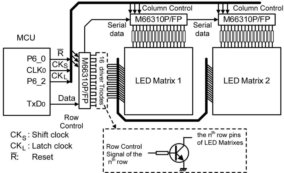
Figure 4.1 Hardware Structure of Application
