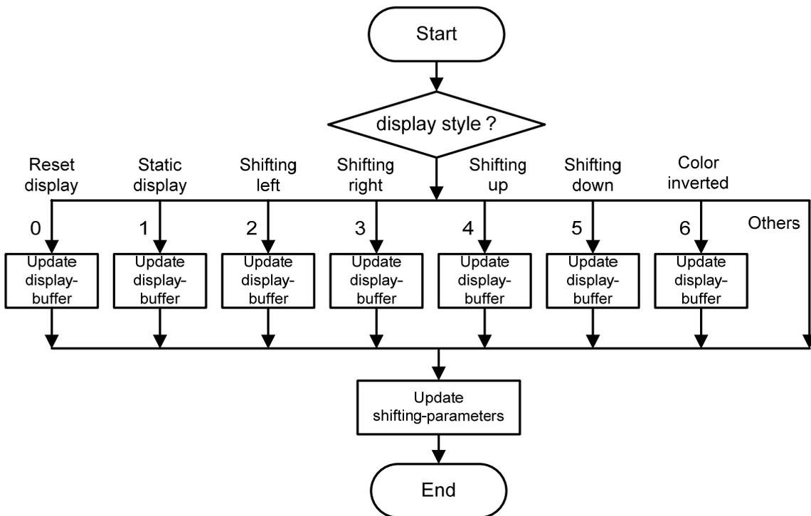
(b) Flow Chart of Updating Display-buffer Sub Function
