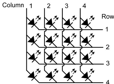
Figure 3.1 A Sample Structure of a Unicolor 4×4 LED Matrix
