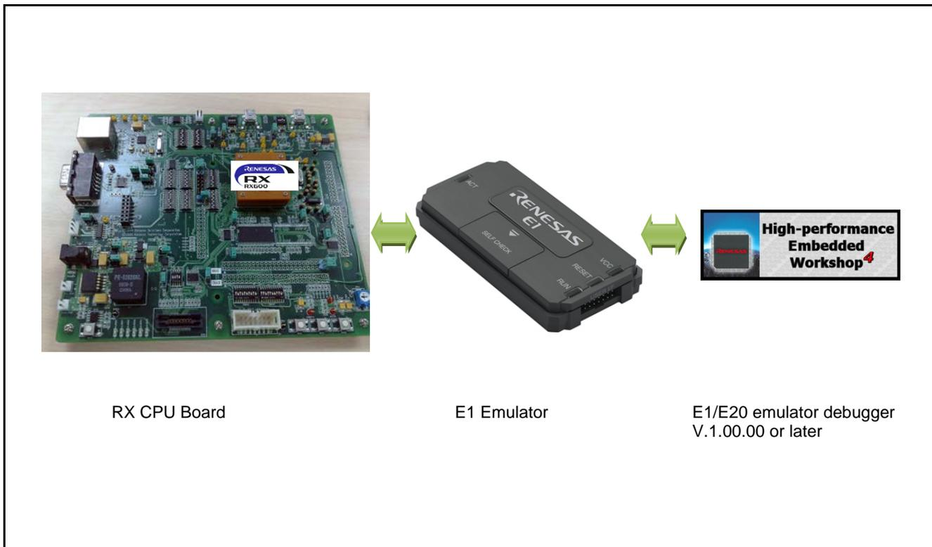
Figure 1 Configuration of the System Used in the Document
