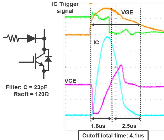
Figure 2-2 DESAT Operation
