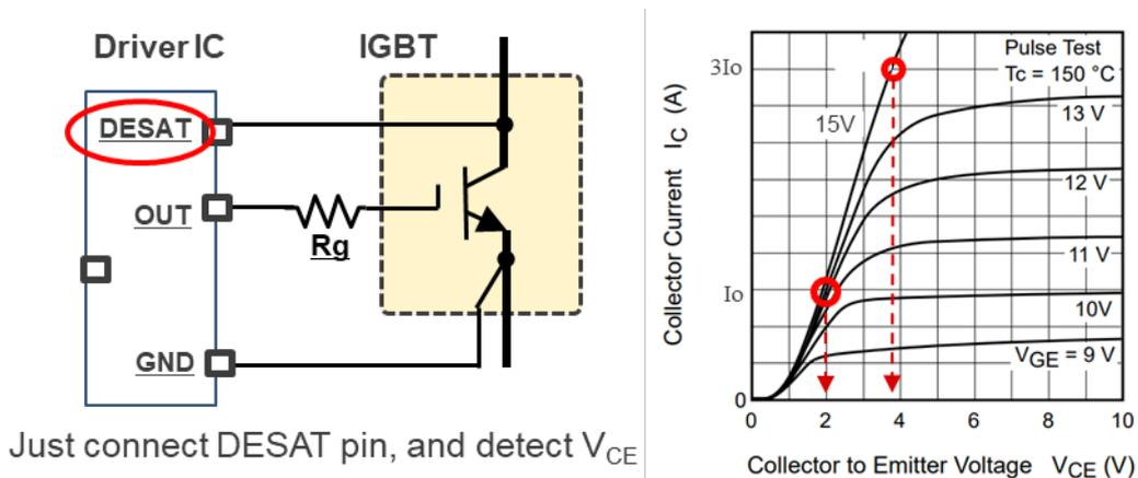
Figure 2-1 DESAT circuit diagram and VCE example value
