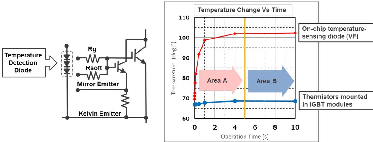
Figure 3-2 Temperature monitoring on different solution
