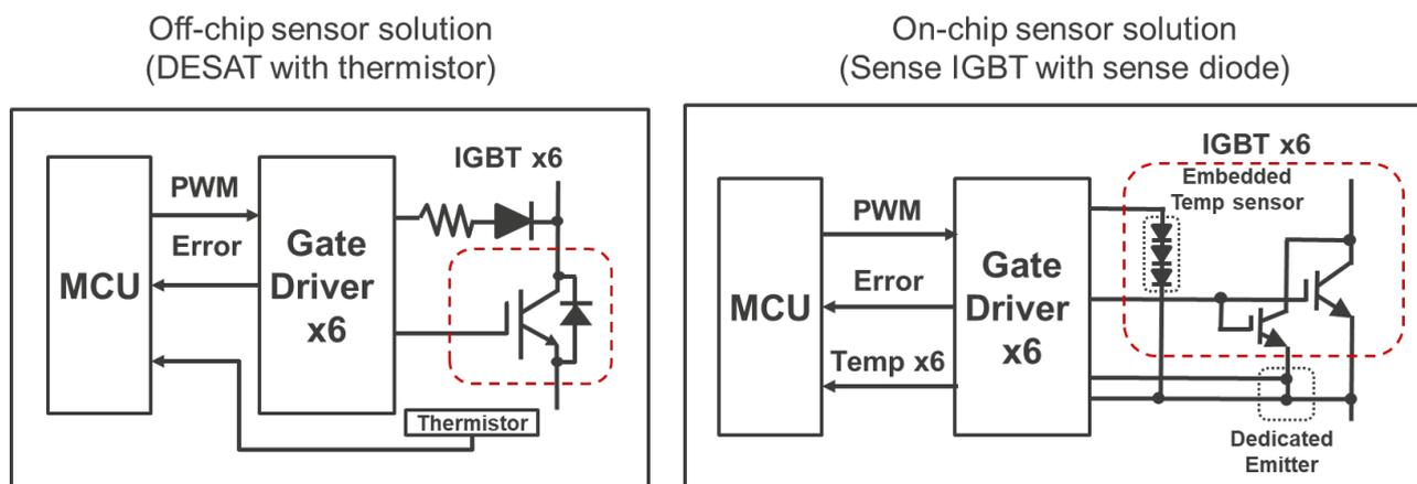
**Figure 5-1 Comparison of On-chip sensor vs Off-chip sensor**
