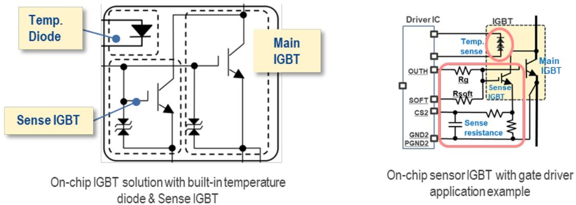
Figure 4-1 IGBT On-chip solution with application example
