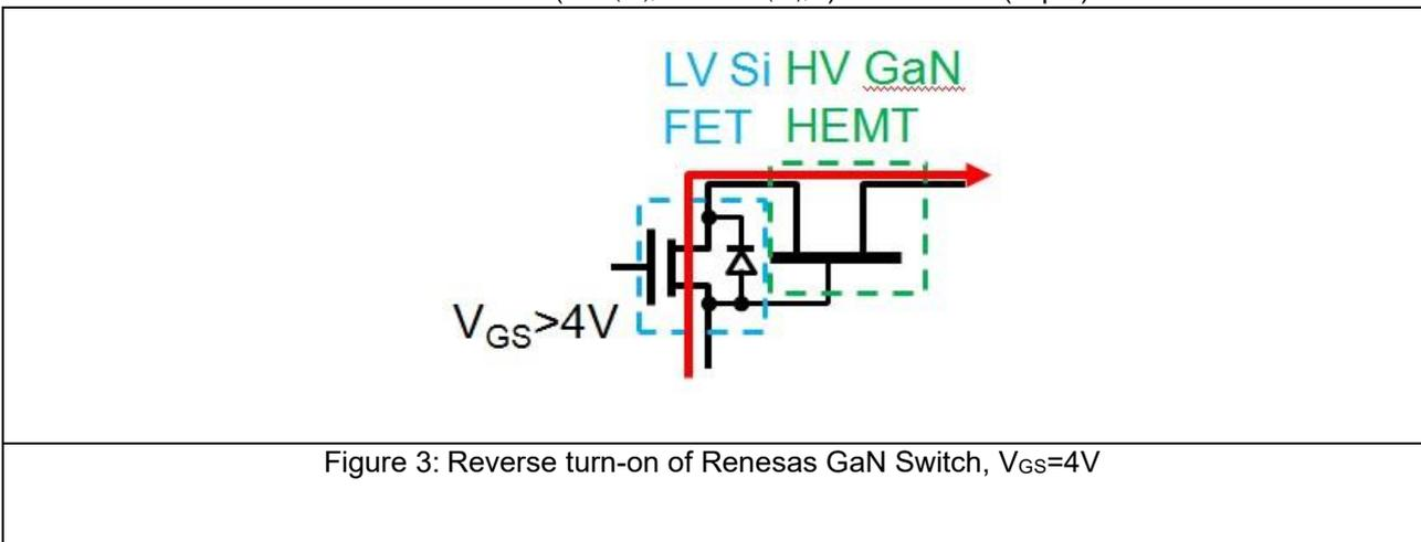
Figure 3: Reverse turn-on of Renesas GaN Switch,  $V_{GS} = 4V$
