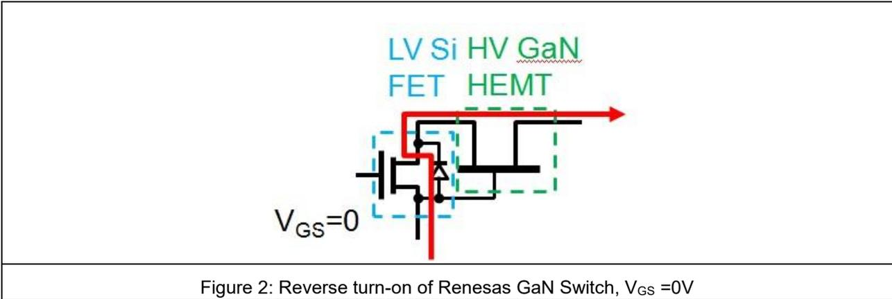
Figure 2: Reverse turn-on of Renesas GaN Switch,  $V_{GS} = 0V$
