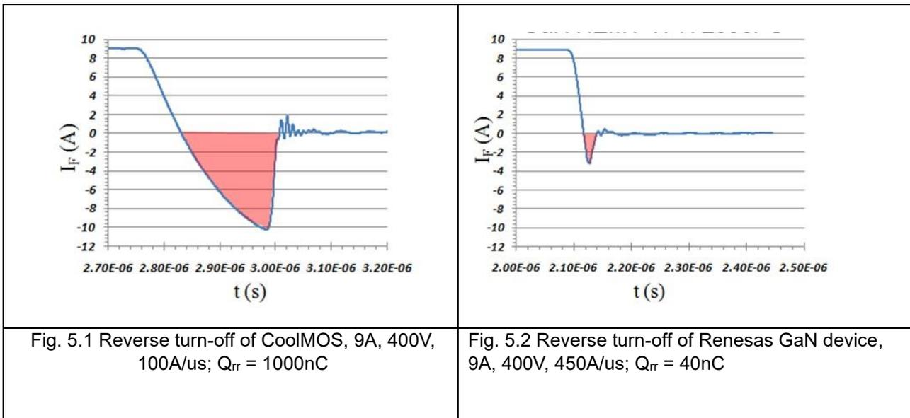
To further analyze the reverse recovery charge of the GaN switch, the reverse recovery charge can be split into two components: First, the capacitive charge of the GaN HEMT, and second, the reverse recovery charge of the low voltage Si MOSFET.
