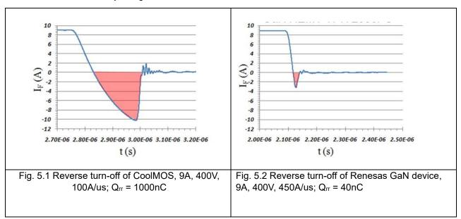
To further analyze the reverse recovery charge of the GaN switch, the reverse recovery charge can be split into two components: First, the capacitive charge of the GaN HEMT, and second, the reverse recovery charge of the low voltage Si MOSFET.
