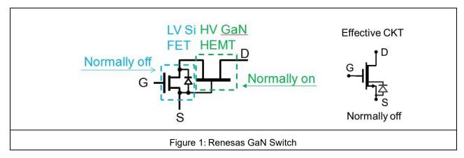
Packaged in this configuration, the Si MOSFET and the GaN HEMT together behave as a single transistor- the GaN switch. The gate and the source of the GaN switch are given by the gate and the source of the Si MOSFET, while the drain of the GaN switch is given by the drain of the
