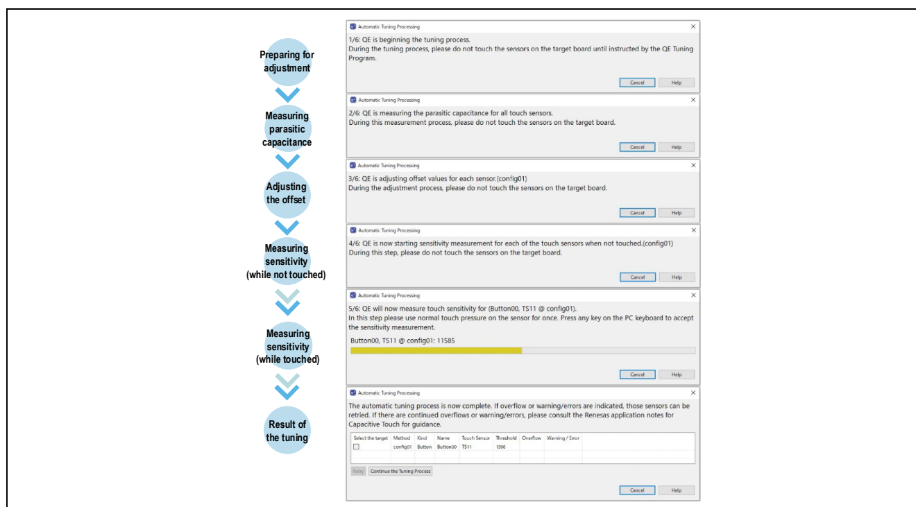
Figure 7.2 Auto tuning using QE for Capacitive Touch
