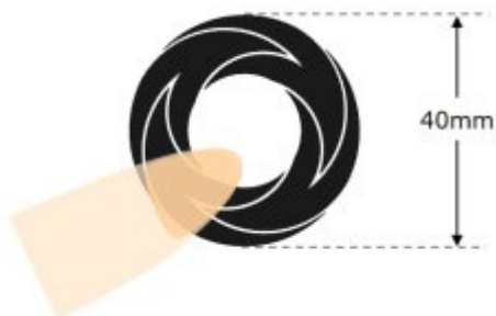
Figure2-29. Recommended Pattern for Wheel Electrode for Self-Capacitance Method
