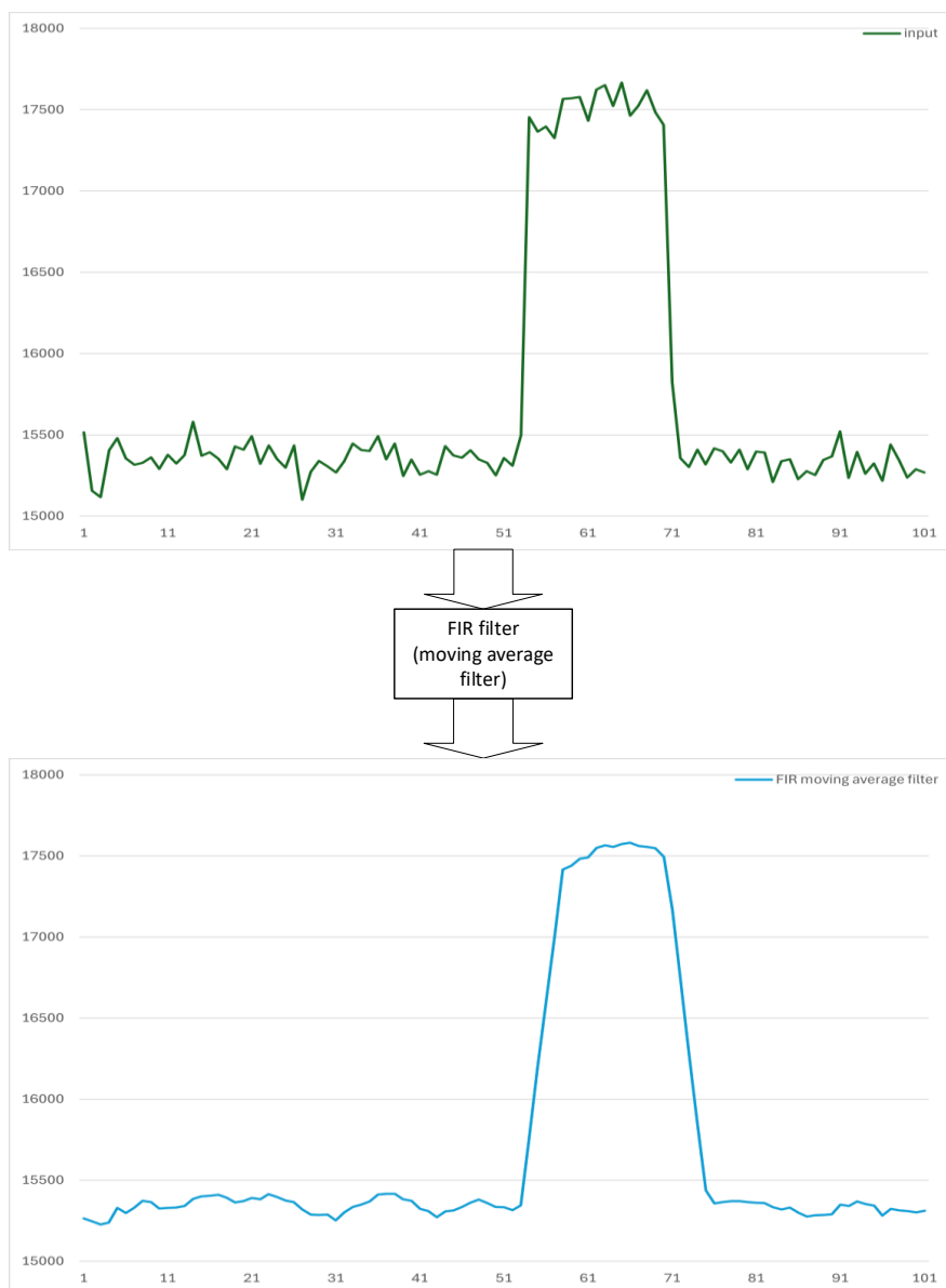
Figure 3-1 FIR Filter Operation (moving-average filter)
