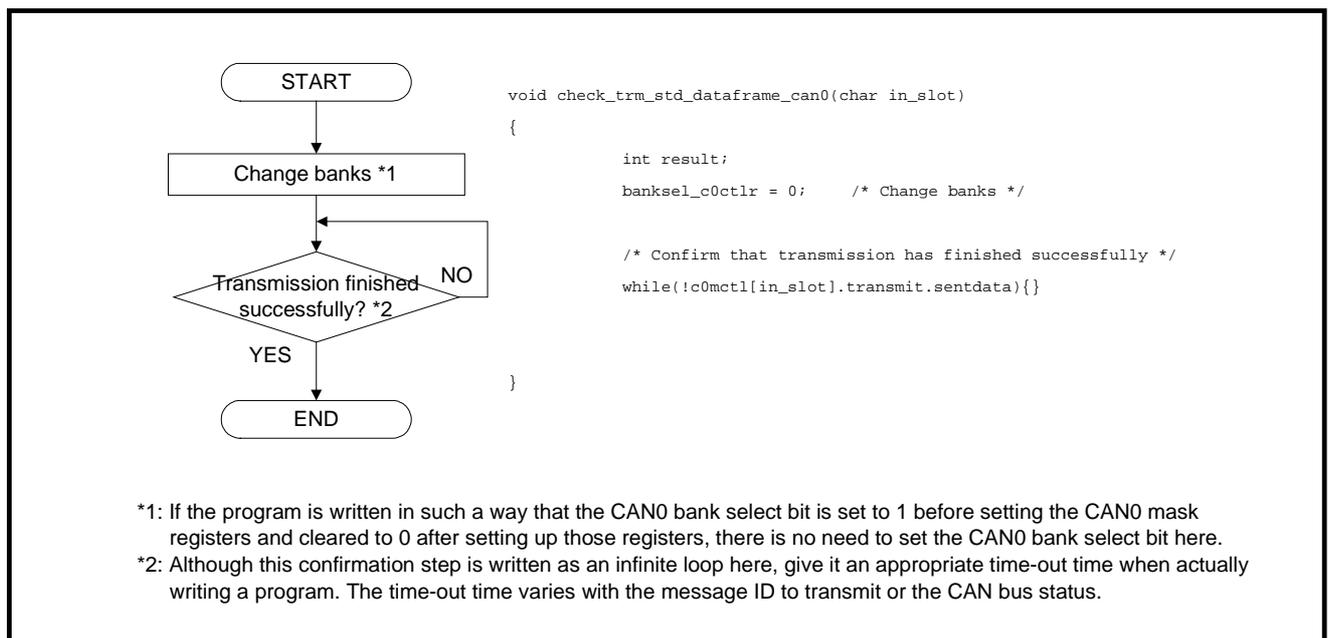
**Figure 3. Confirming procedure of a successful transmission by polling**
