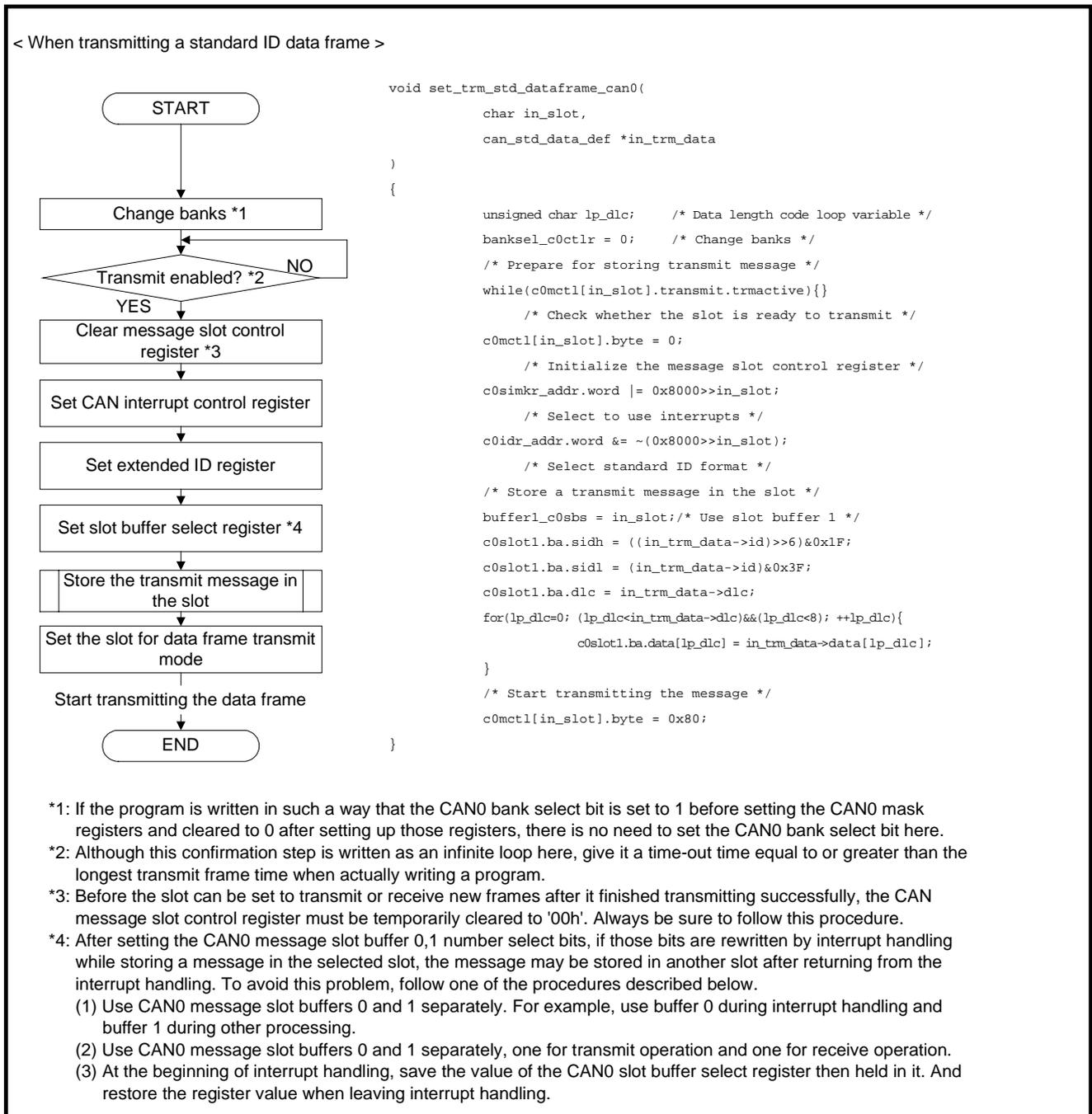
Figure 2. Transmitting procedure of a data frame
