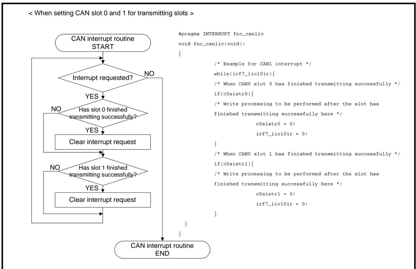
**Figure 4. Confirming procedure of a successfully transmission by using CAN interrupt**
