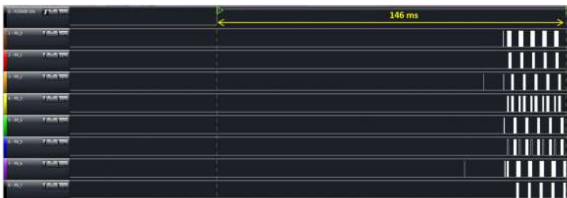
Figure 4: DA14580: Scan timing for booting from external serial devices
