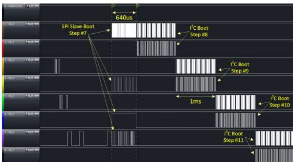
Figure 9: SPI Slave and I2C boot timing
