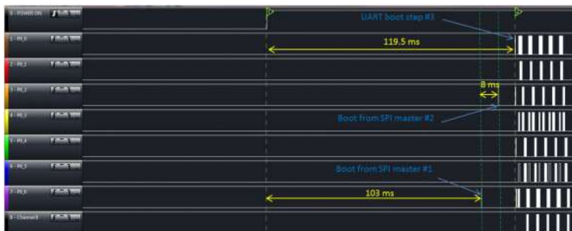
Figure 6: DA14580: Boot timing from SPI Master
