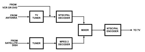
FIGURE 1. TYPICAL VIDEO PATH OF SATELLITE DIGITAL SETTOP BOX
