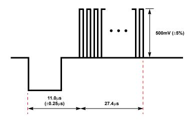
FIGURE 1. 625-LINE WSS LINE 23 TIMING
