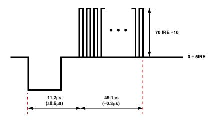
FIGURE 2. 525-LINE WSS LINE 20 AND LINE 283 TIMING
