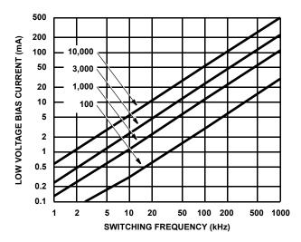
FIGURE 9. LOW VOLTAGE BIAS CURRENT I<sub>DD</sub> AND I<sub>CC</sub> (LESS QUIESCENT COMPONENT) vs FREQUENCY AND GATE LOAD CAPACITANCE
