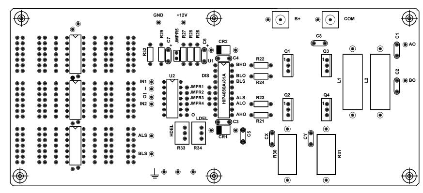
FIGURE 13. HIP4080A/81AEVALZ EVALUATION BOARD SILKSCREEN
