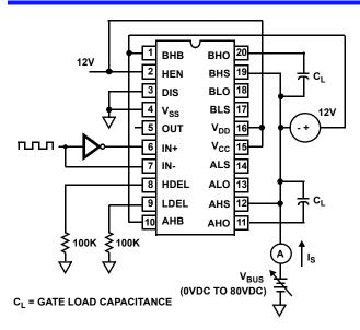
FIGURE 10. HIGH VOLTAGE LEVEL-SHIFT CURRENT TEST
