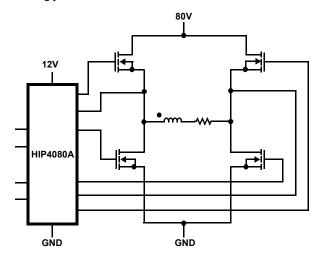
FIGURE 1. HIP4080A SIMPLIFIED APPLICATION DIAGRAM
