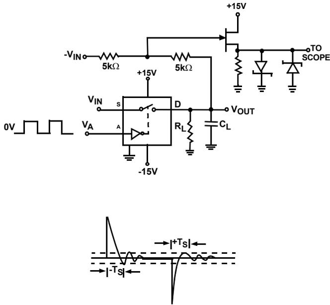
SETTLING TIME ( $T_S$ ) IS MEASURED USING A HIGH SPEED RECOVERY OSCILLOSCOPE TO DISPLAY THE ERROR VOLTAGE  $V_E$ .
