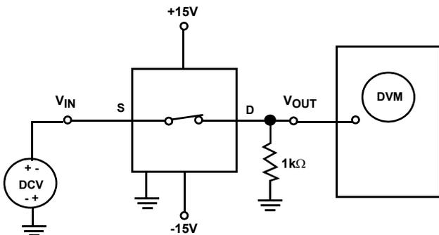
FIGURE 1. SUGGESTED CIRCUIT TO DETERMINE ANALOG SIGNAL RANGE
