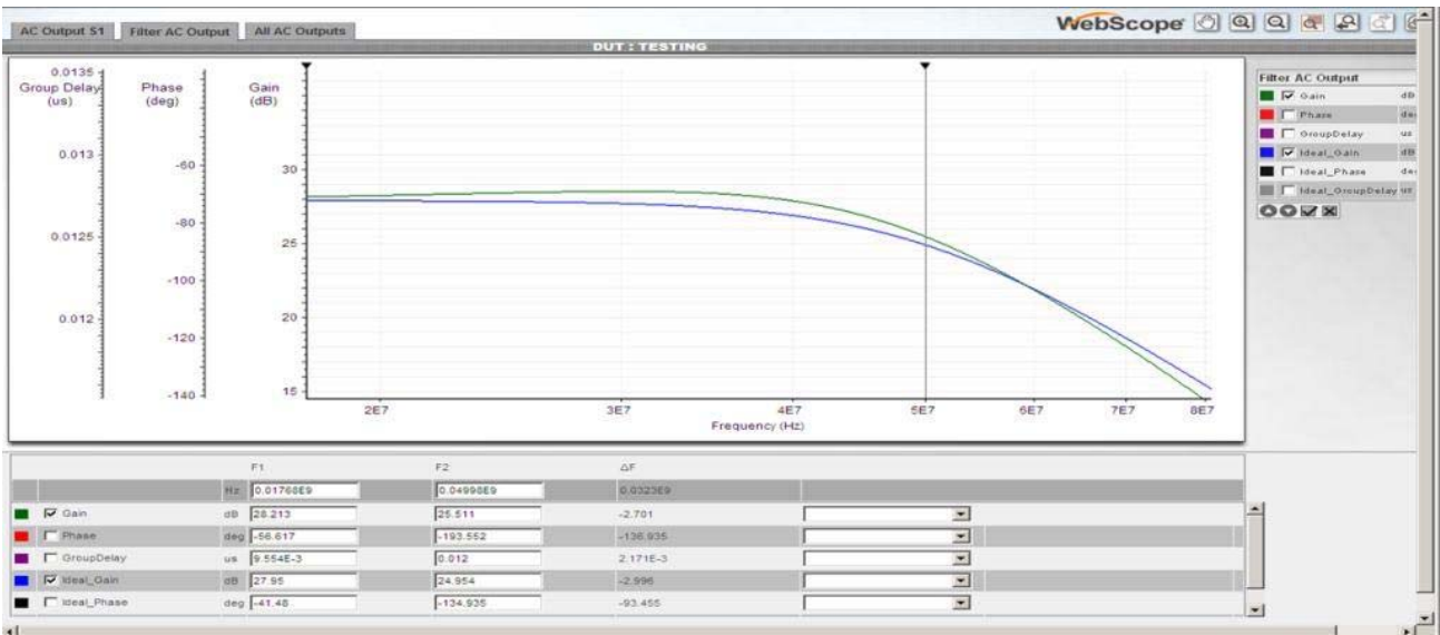
FIGURE 58. COMPARISON OF SIMULATED TO IDEAL GAIN RESPONSE
