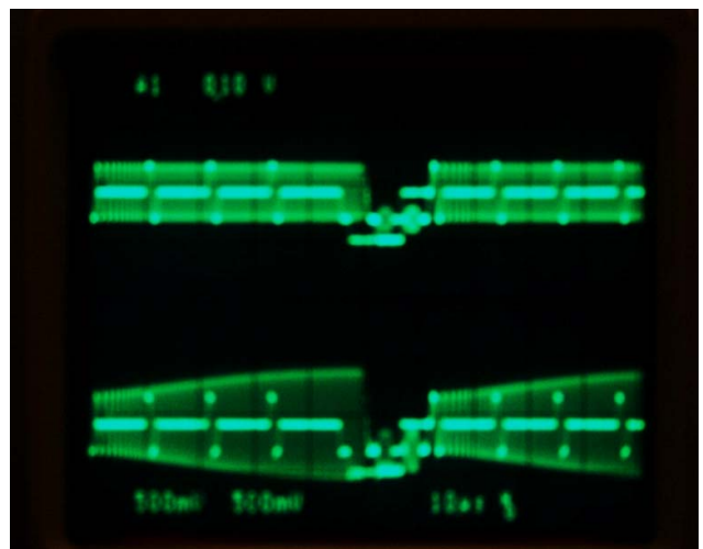
FIGURE 25. CABLE COMP AT MAXIMUM - VIDEO GAIN AT MINIMUM DCP SETTINGS
