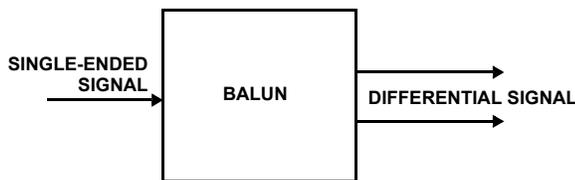
FIGURE 1. BLOCK DIAGRAM OF A BALUN
