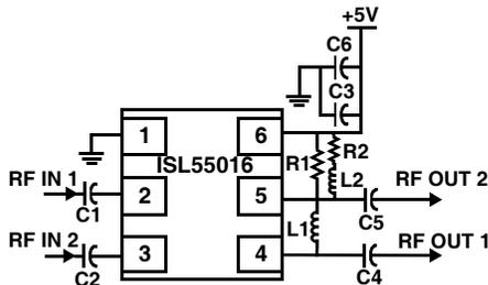
FIGURE 2. APPLICATION CIRCUIT
